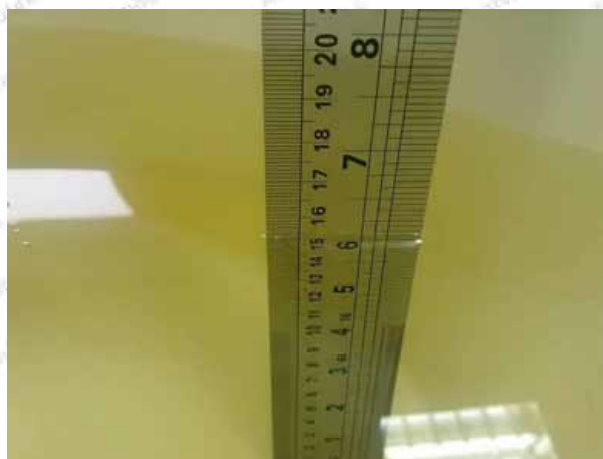
Photograph of the depth in the Phantom(900MHz)
