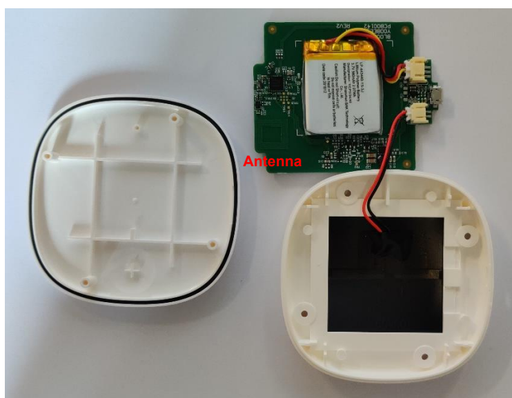
Figure 4: inside view PCB front with connection to the plastics
