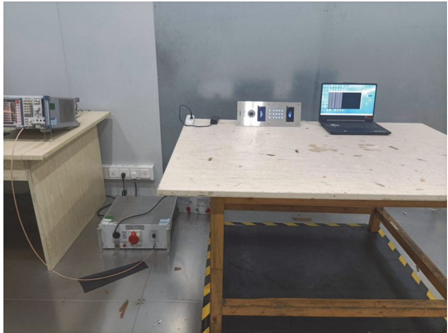
Conducted Emission Test Setup
