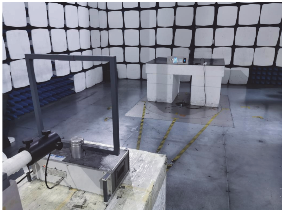
Radiation Emission Test Setup (Below 30MHz)
