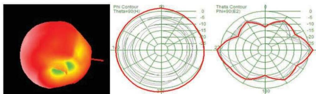
433.92MHz Peak Gain: 0 dBi Efficiency: 50.1%
