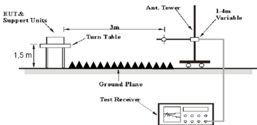
The radiated emission below 1GHz tests were performed in the 3 meters chamber A, above 1GHz tests were performed in the 3 meters chamber B, using the setup accordance with the ANSI C63.10-2013. The specification used was the FCC 15.209, and FCC 15.247 limits.
