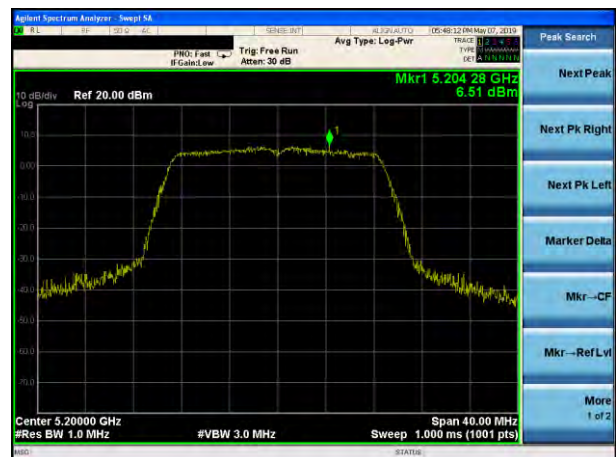
(802.11n20) PSD plot on channel 40
