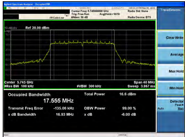
(802.11 n20) 6dB Bandwidth plot on channel 149
