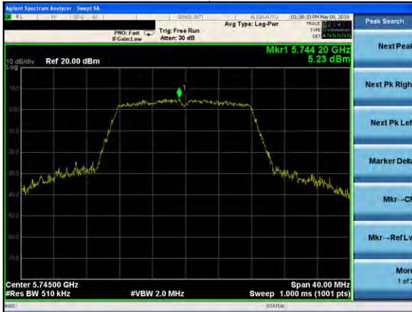
(802.11a) PSD plot on channel 157
