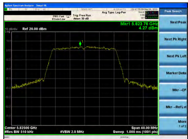
(802.11ac20) PSD plot on channel 165
