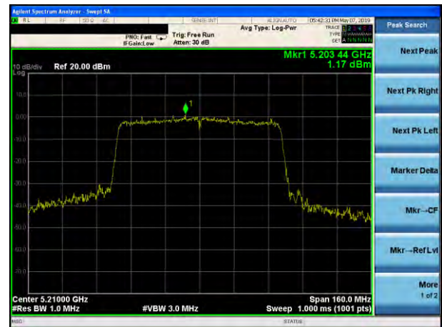
(802.11ac80) PSD plot on channel 42
