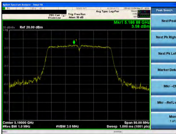
(802.11ac40) PSD plot on channel 38
