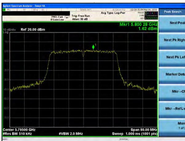
(802.11n40) PSD plot on channel 159
