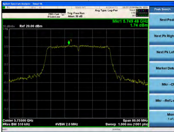
(802.11ac40) PSD plot on channel 159
