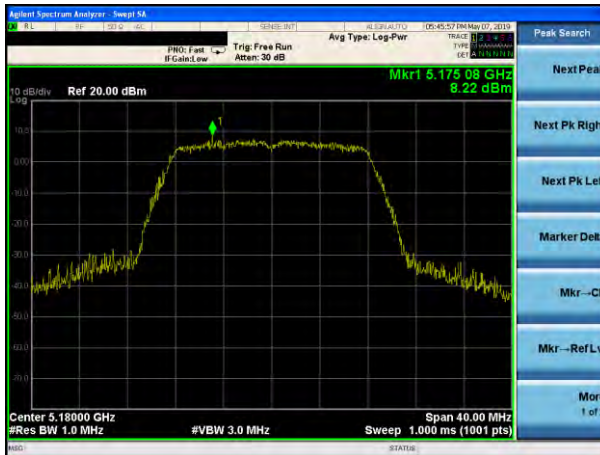
(802.11a) PSD plot on channel 36
