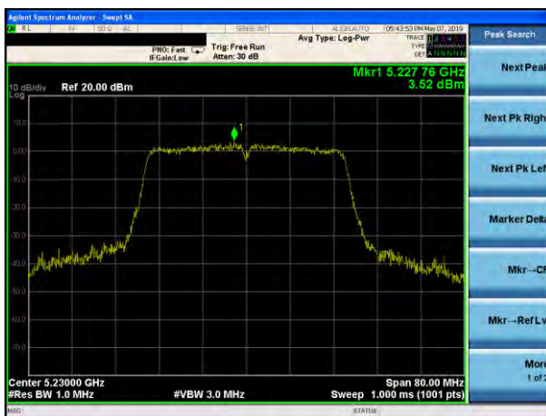
(802.11ac40) PSD plot on channel 46
