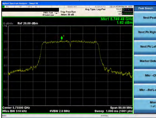
(802.11n40) PSD plot on channel 159
