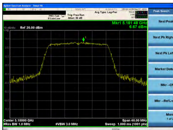
(802.11ac20) PSD plot on channel 36
