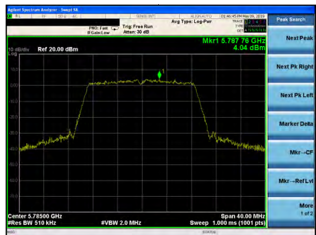
(802.11ac20) PSD plot on channel 165
