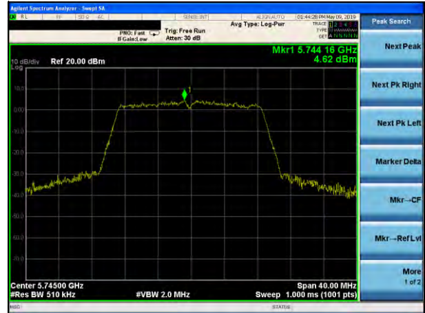
(802.11n20) PSD plot on channel 157
