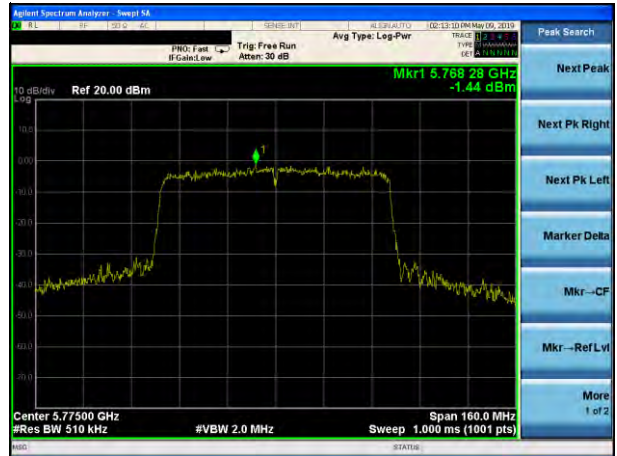
(802.11ac80) PSD plot on channel 155
