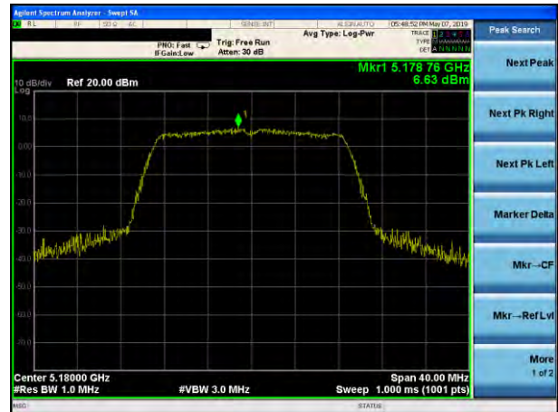
(802.11n20) PSD plot on channel 36
