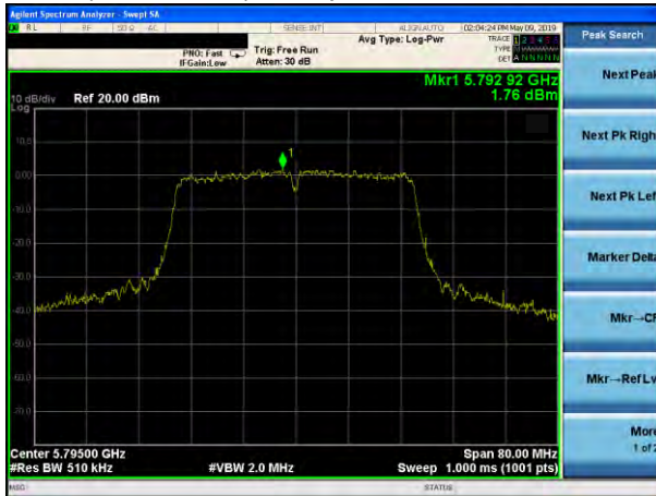
(802.11ac40) PSD plot on channel 159
