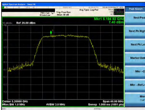
(802.11a) PSD plot on channel 40
