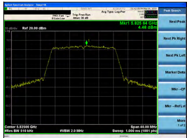
(802.11n20) PSD plot on channel 165
