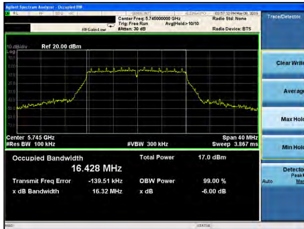
(802.11a) 6dB Bandwidth plot on channel 149
