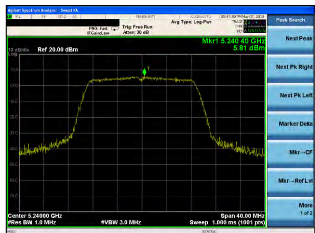
(802.11n20) PSD plot on channel 48
