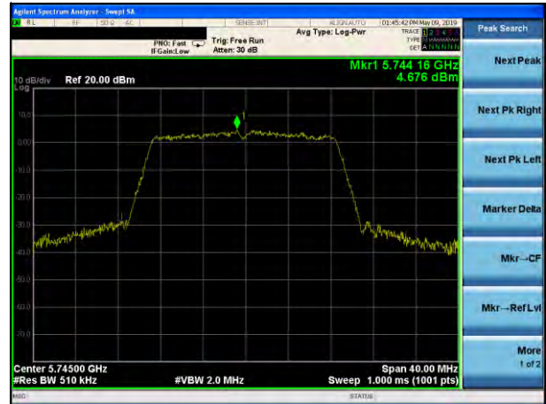
(802.11ac20) PSD plot on channel 157
