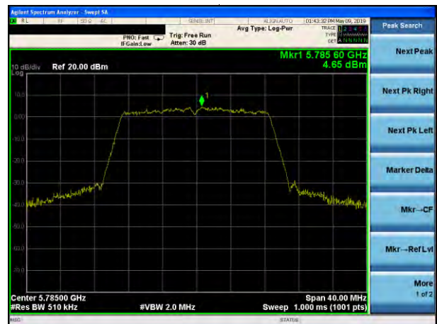
(802.11n20) PSD plot on channel 165
