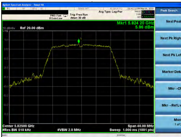
(802.11a) PSD plot on channel 165
