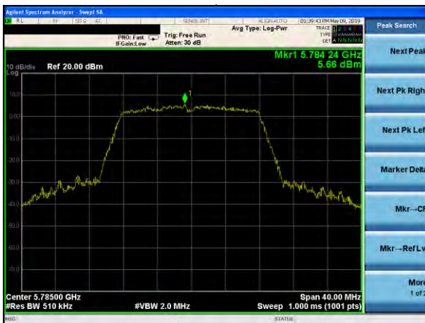
(802.11a) PSD plot on channel 165
