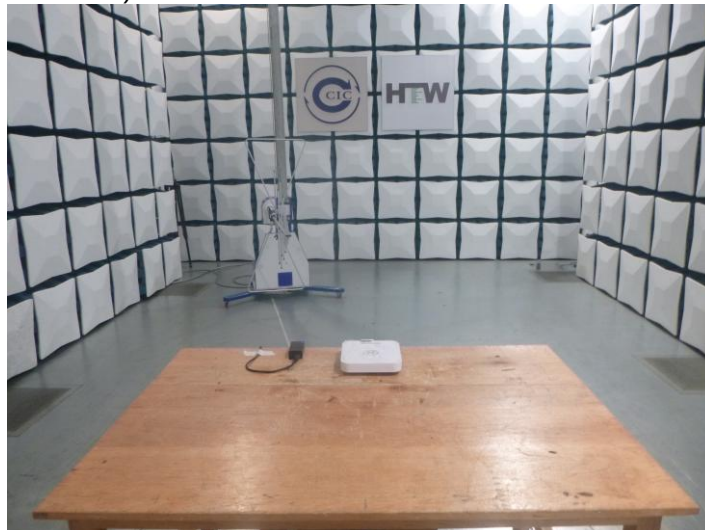
Radiated Emissions (30MHz-1GHz)
