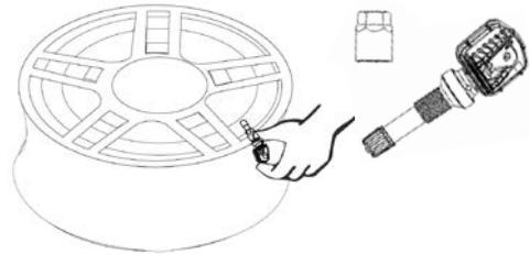
1.3 Take off the nut<sup>④</sup>, insert the valve stem through the rim hole from inside.
