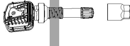
1.4 Place nut<sup>④</sup> on the valve stem, and tighten with 5 Nm (44 inch pounds) torque.
