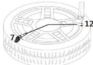
1.6 Mount the upper tyre bead the same way. (If the mounting head of the tyre changer is positioned at 12 o'clock, then the valve should be at the 5 o'clock position.) Inflate the tyre to nominal pressure.
