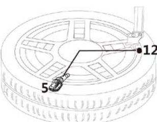
1.7 Apply soapsuds on the valve tip. If no leakage is found, put on the valve cap<sup>⑥</sup>. If unsuccessful, try again.
