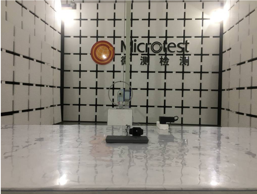
Radiated emission(Watch: 30MHz-1GHz)
