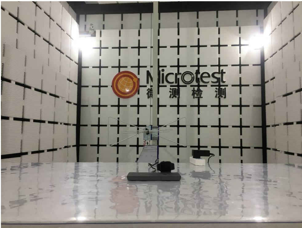
Radiated emission(Watch: 30MHz-1GHz)
