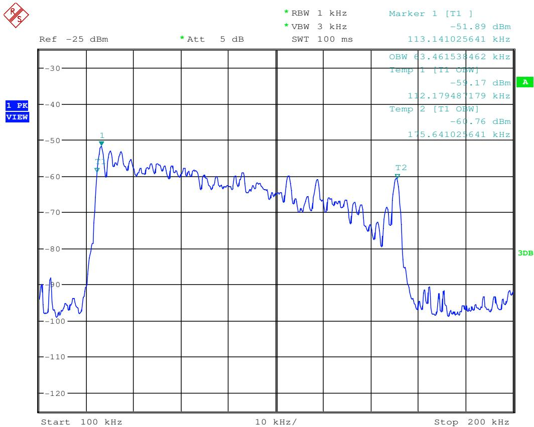
According the test data above, the fundamental wave is not fall in the restricted band 90KHz-110KHz, the field strength also meet the 15.209 requirement, please refer to clause 7.4.
