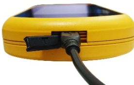
Fig 8-1 Open the silicone protective plug
