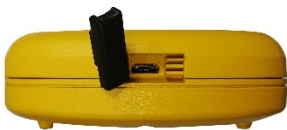
Fig 8-1 Open the silicone protective plug
