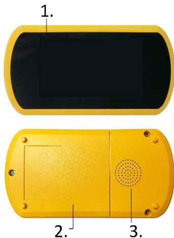
Fig 1-1 Front & rear view of the oximeter
