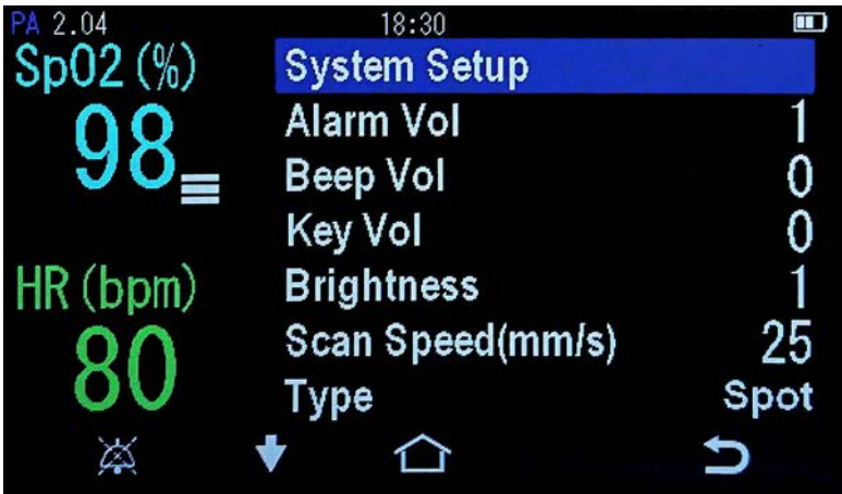
Fig 3-2(a) System setup window
