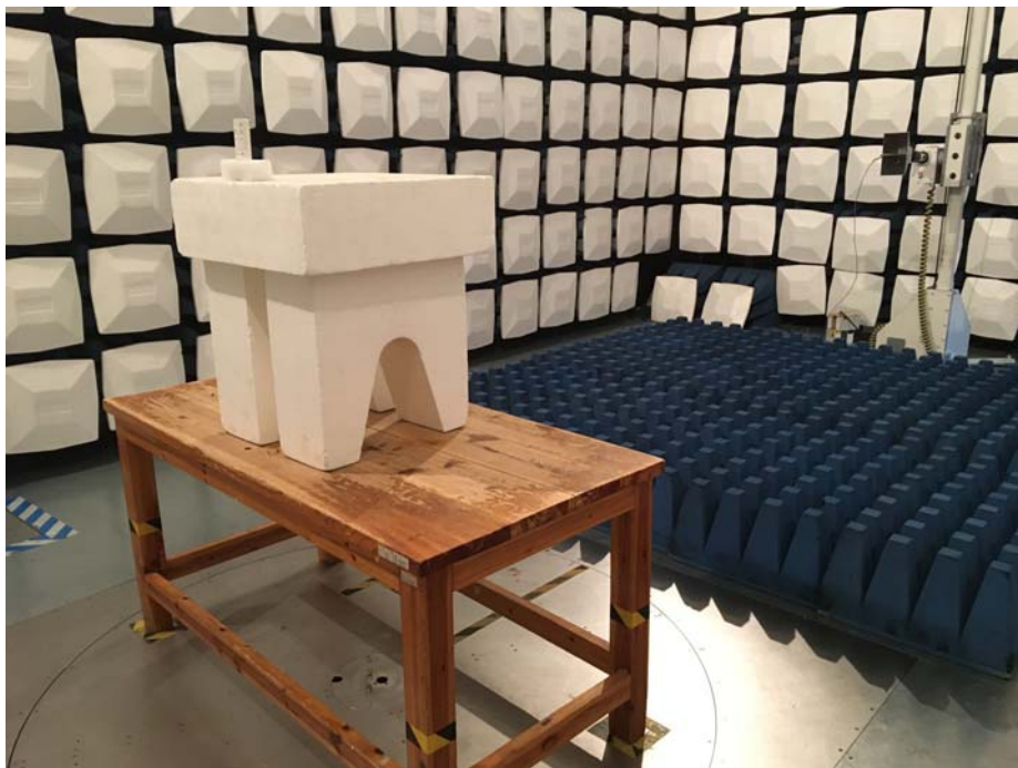
Test Setup For Radiated Emission (Above 1GHz)
