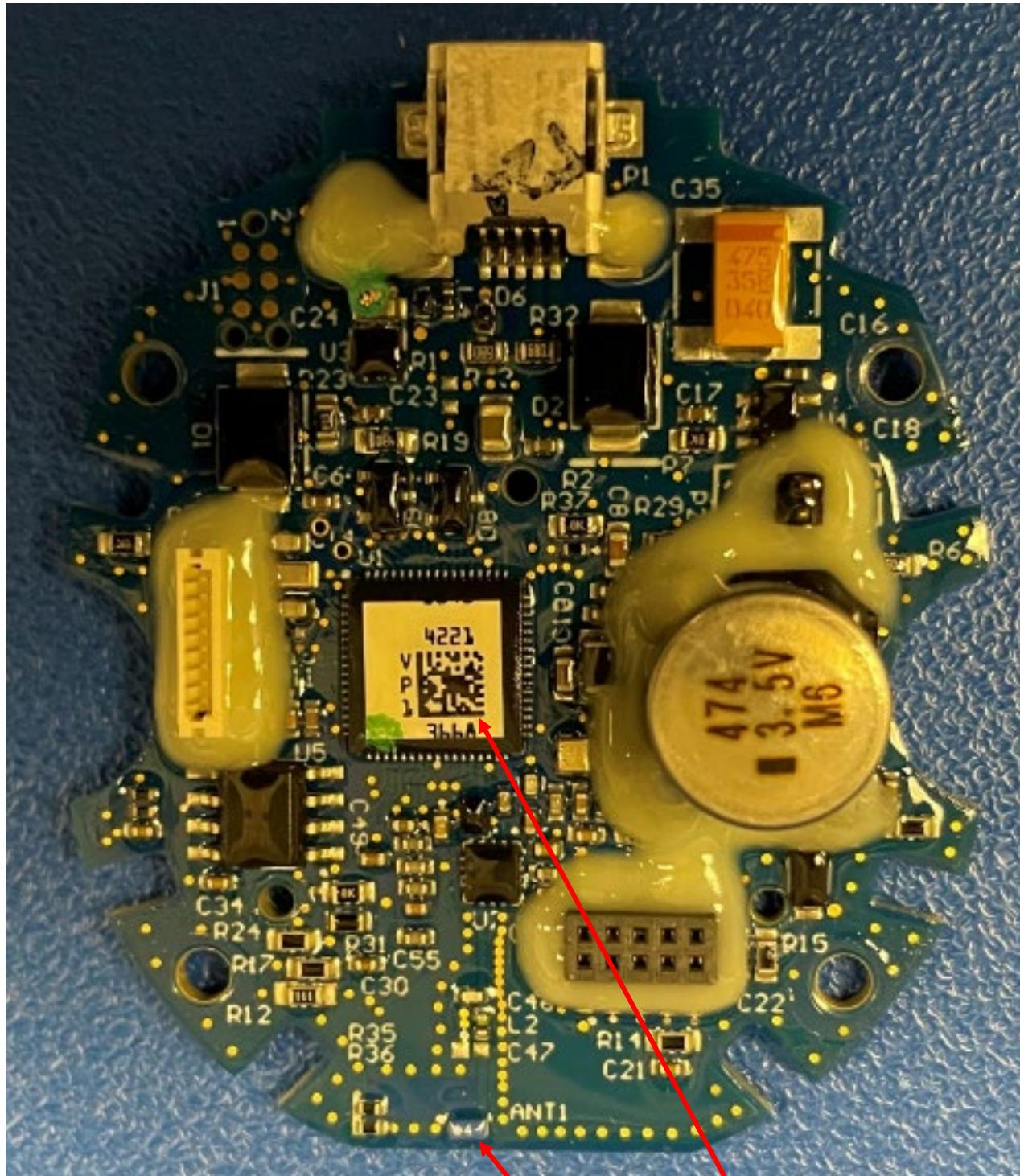
Transmitter, Integrated into MCU
