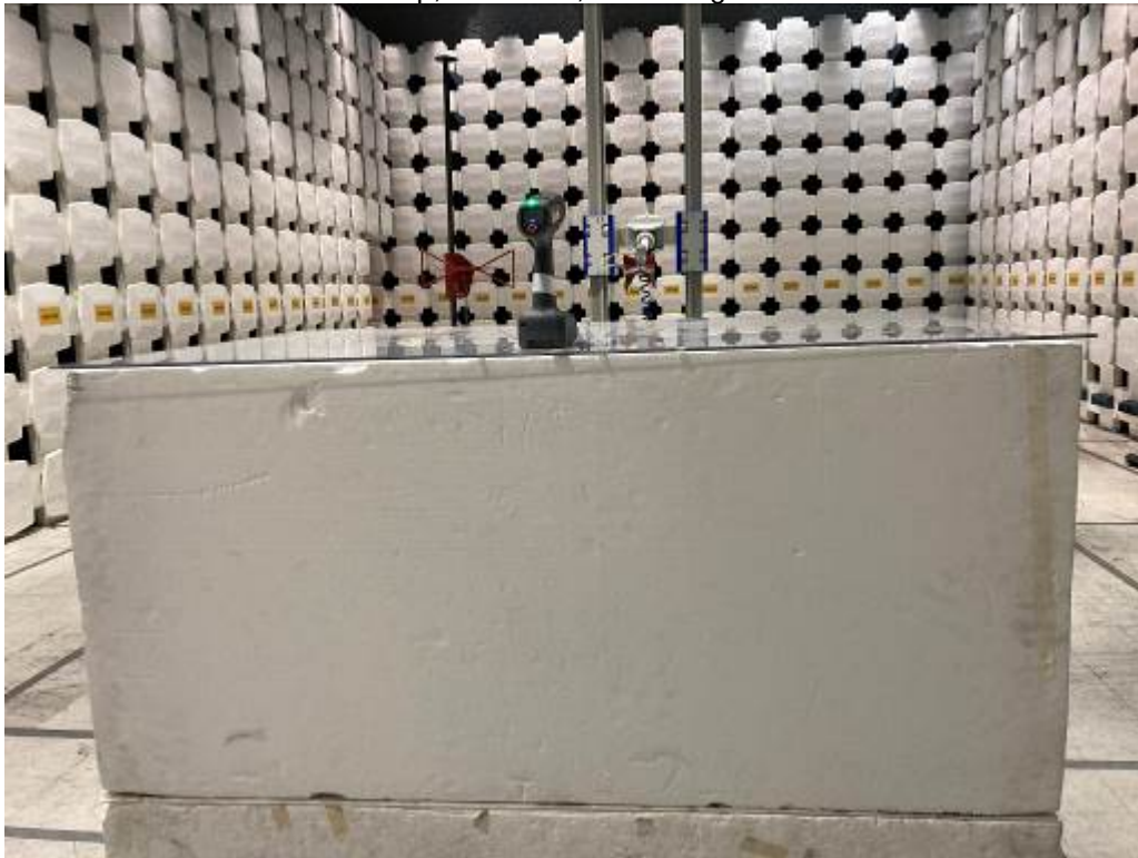
Test Setup, 1-18 GHz, Pistol Angle Wrench
