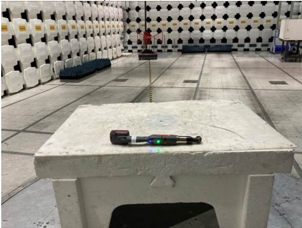
Test Setup, 30-1000 MHz, Low Torque Wrench
