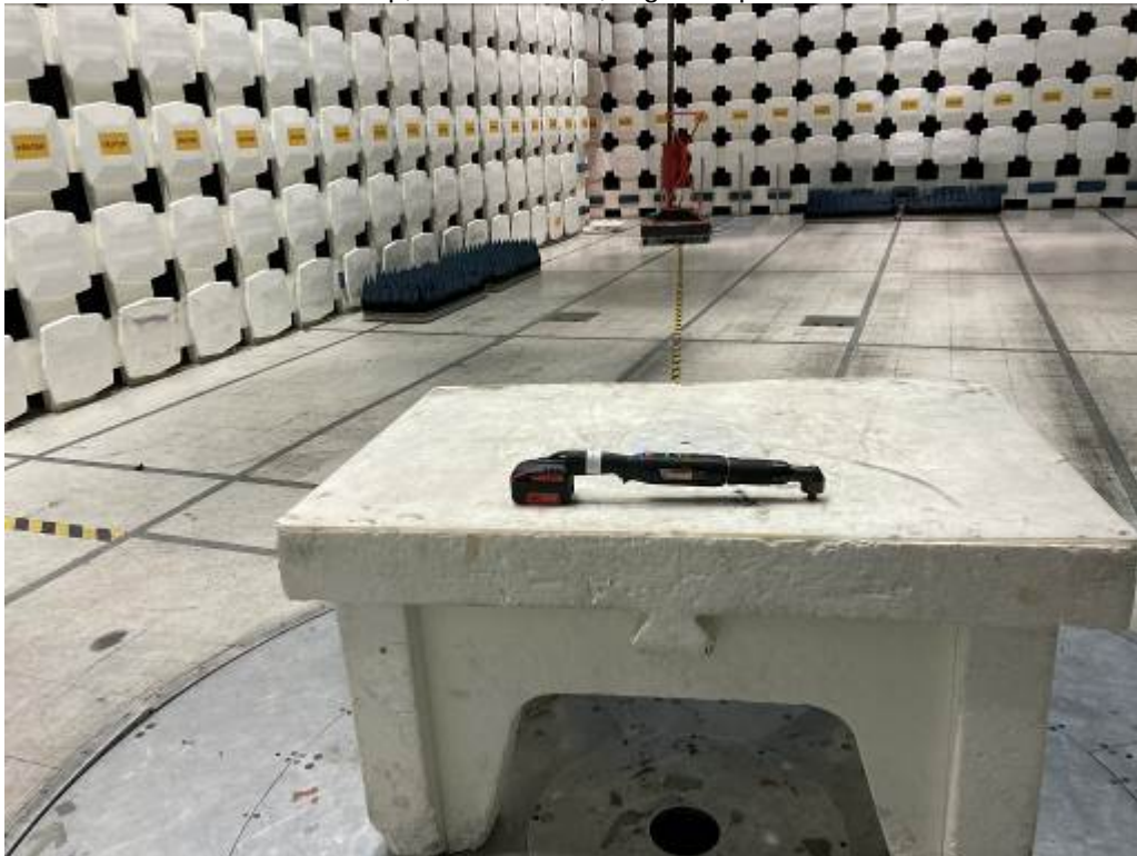
Test Setup, 30-1000 MHz, High Torque Wrench
