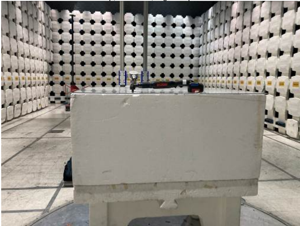
Test Setup, 1-13 GHz, High Torque Wrench
