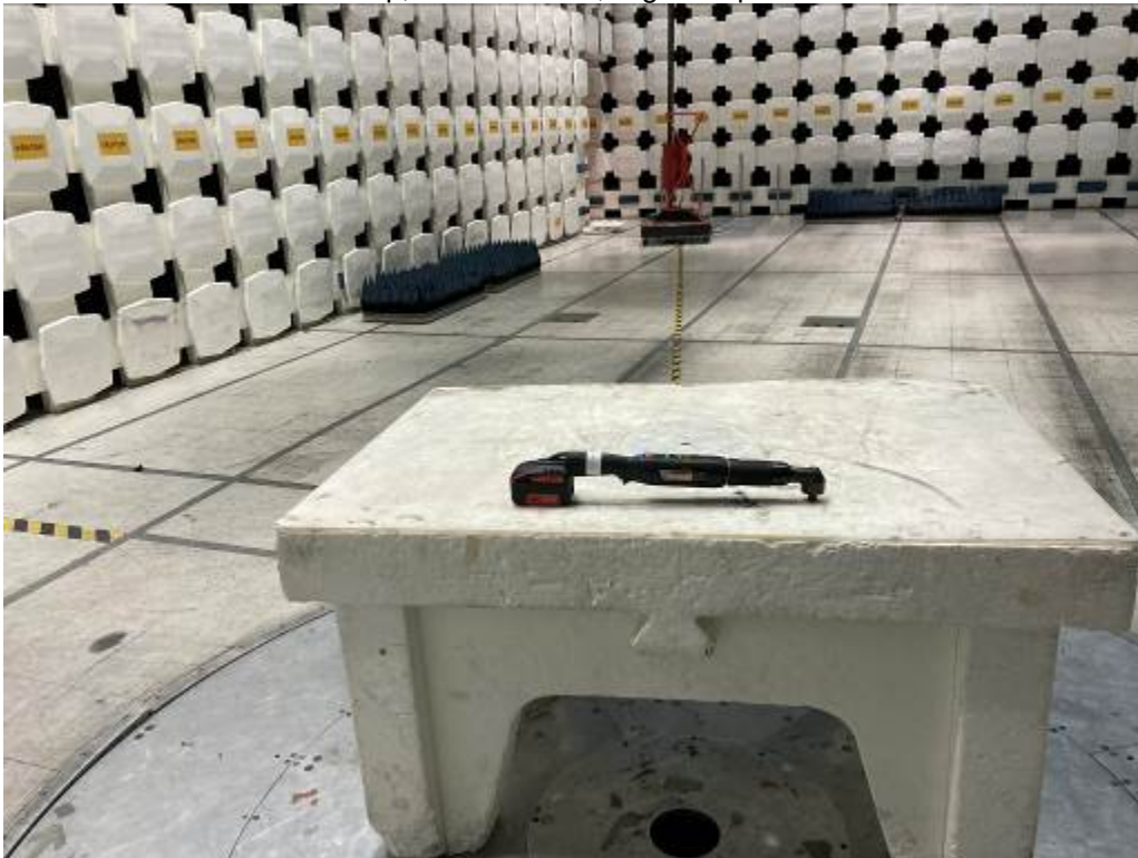
Test Setup, 30-1000 MHz, High Torque Wrench
