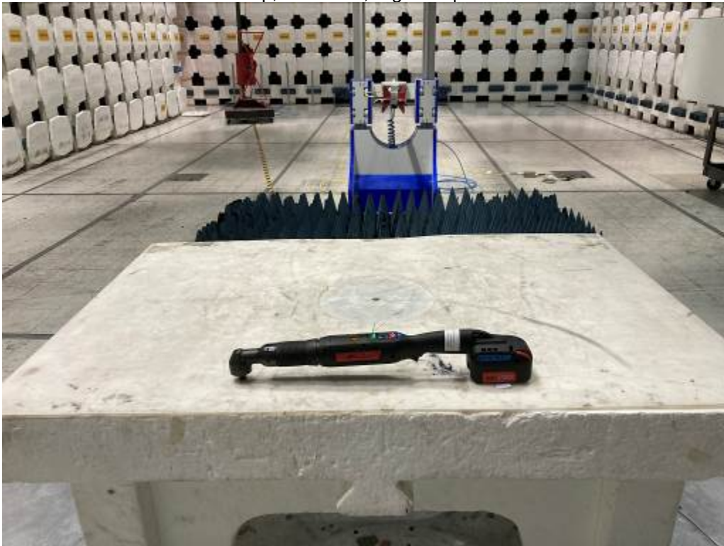
Test Setup, 1-13 GHz, High Torque Wrench
