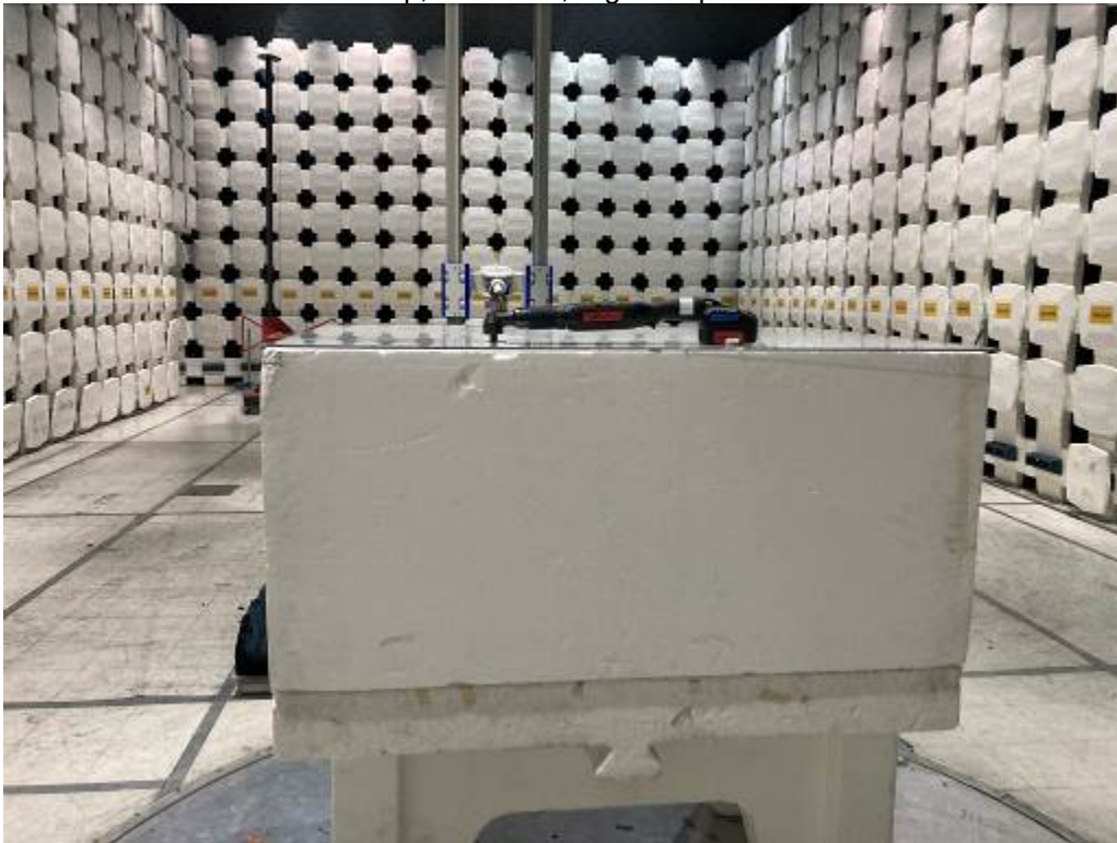
Test Setup, 1-13 GHz, High Torque Wrench
