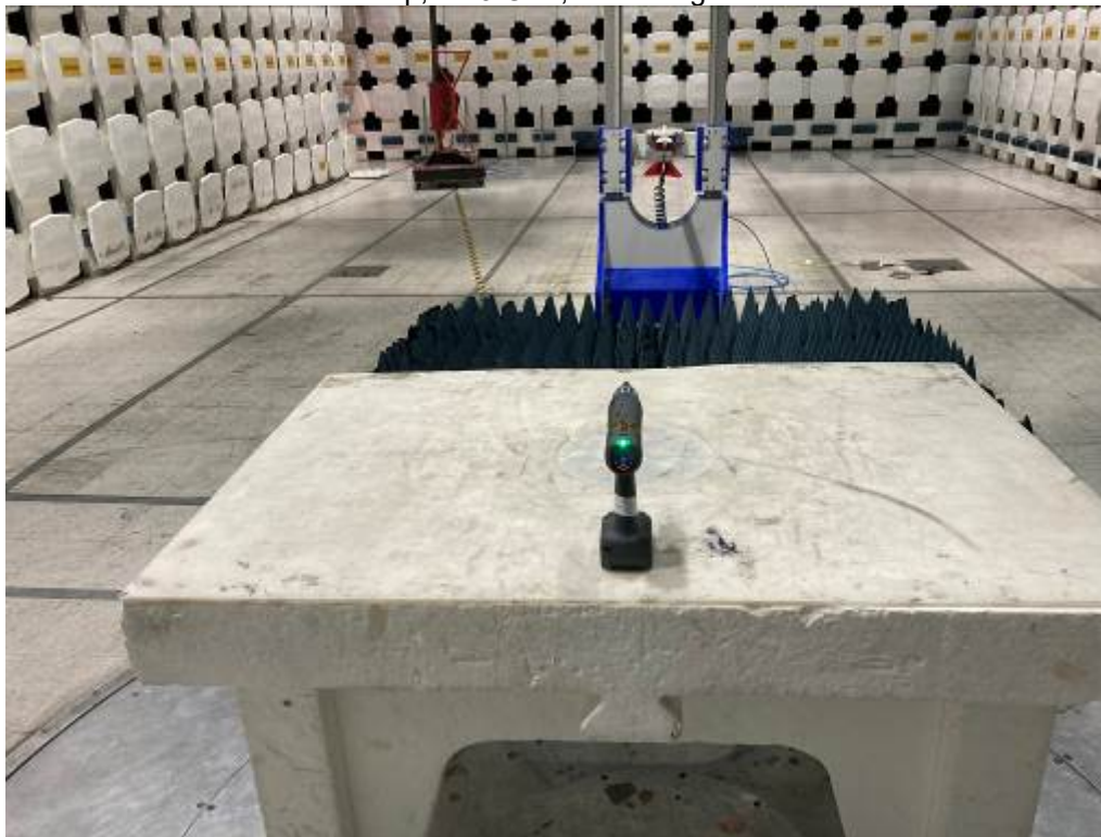
Test Setup, 1-13 GHz, Pistol Angle Wrench
