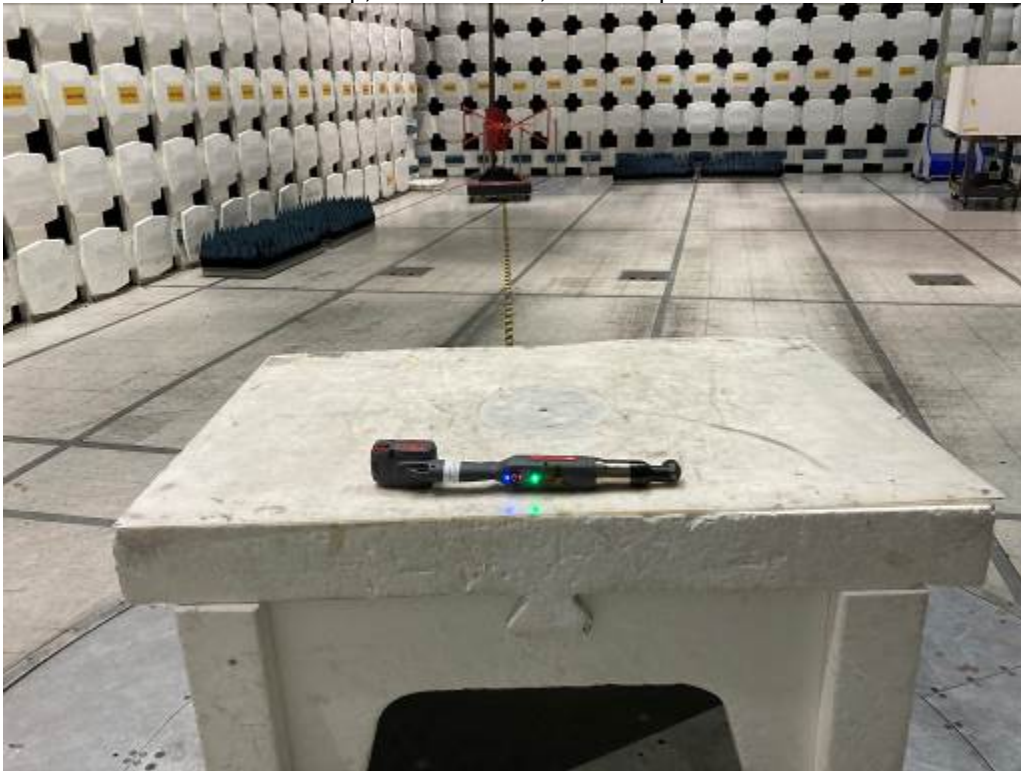
Test Setup, 30-1000 MHz, Low Torque Wrench
