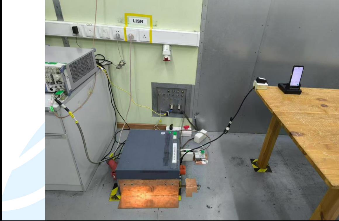
Conducted Emission Test Setup _Test Mode 6
