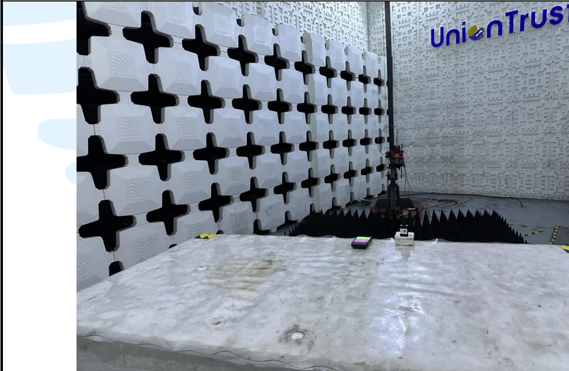
Radiated emission Test Setup (Above 1 GHz) _Test Mode 1
