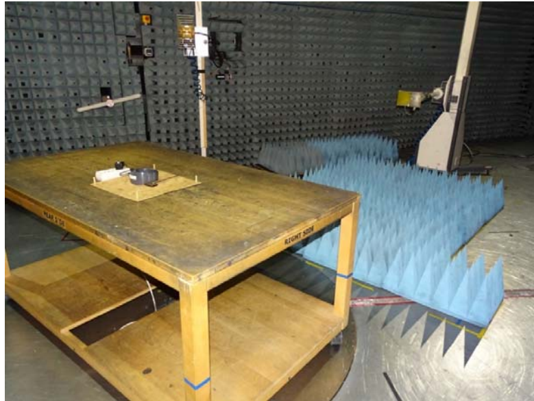
Photo 3: Test setup for radiated measurements above 1 GHz
