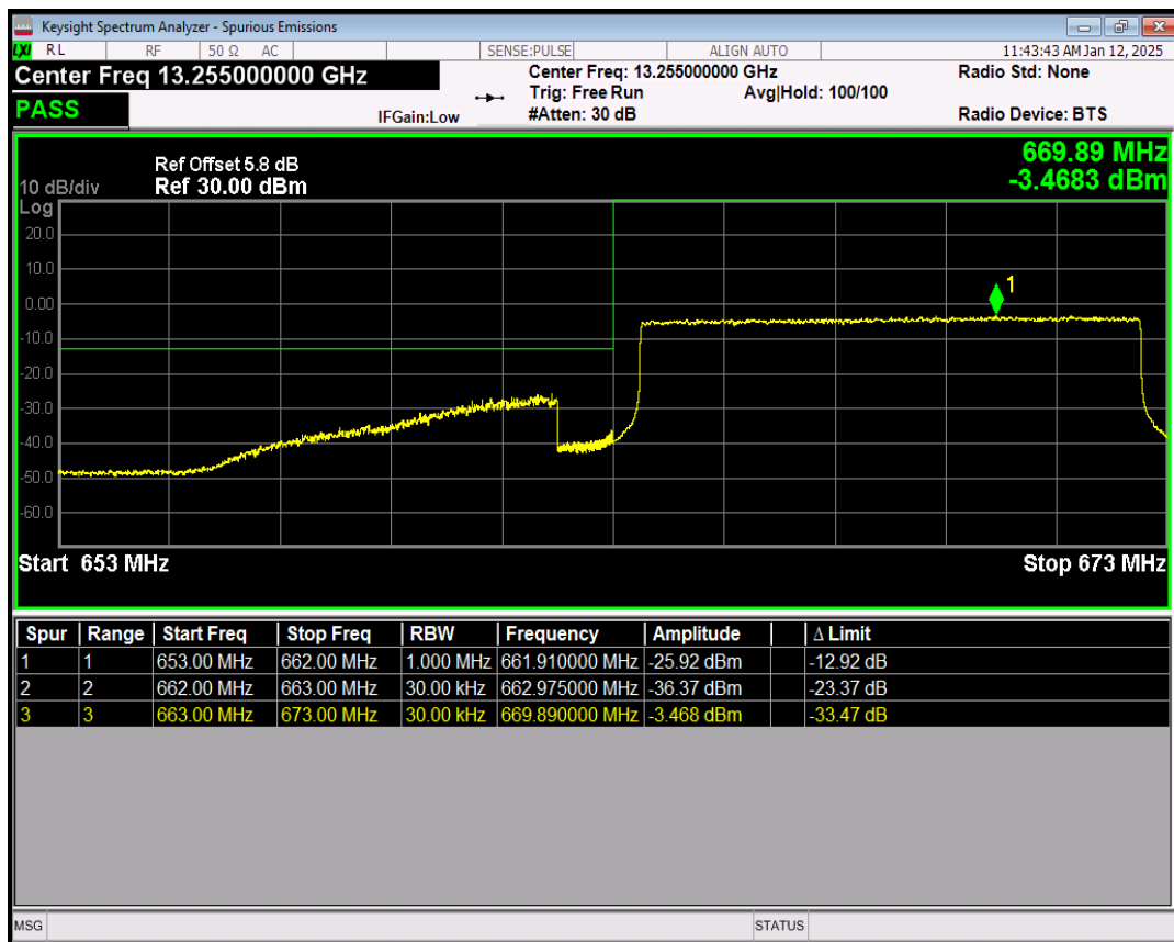
Band71 16QAM BW=10MHz Channel=133172 RB Size=1 Position=#0
