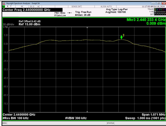
In-Band Reference Level BLE 1M_Channel 19
