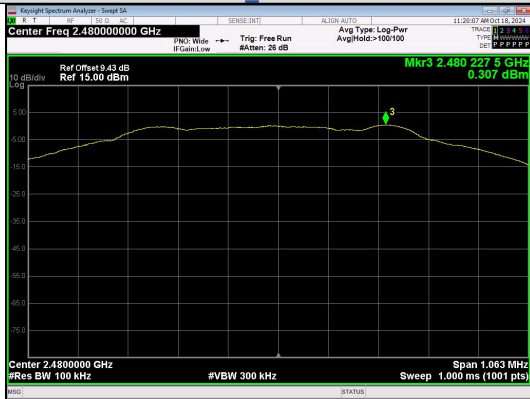
In-Band Reference Level BLE 1M_Channel 39
