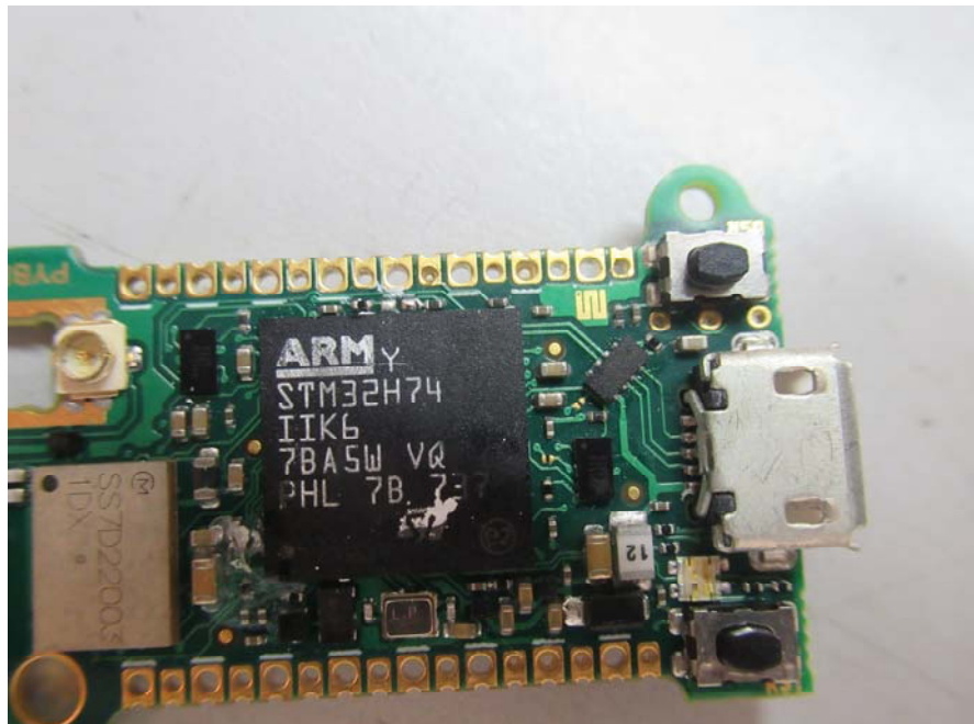
PYBD-SH3W – PCB Chip View
