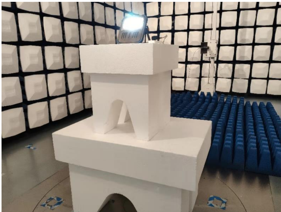
Test Setup For Radiated Emission (Above 1GHz)
