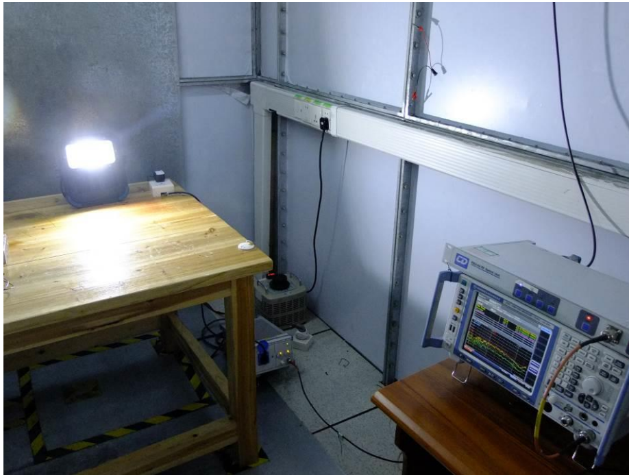
Test Setup For Conducted Emission
