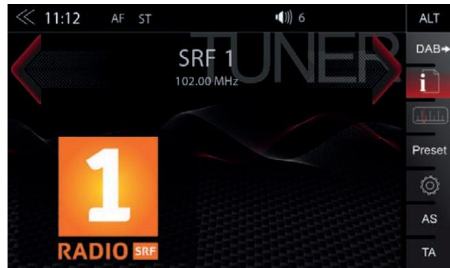
The FM RDS source menu offers a control-/operating section on the right hand side, for fast and convenient adjustments during the FM radio playback.
