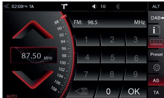
When you tap to the frequency display area, the numeric input keyboard opens for a direct station frequency input.
