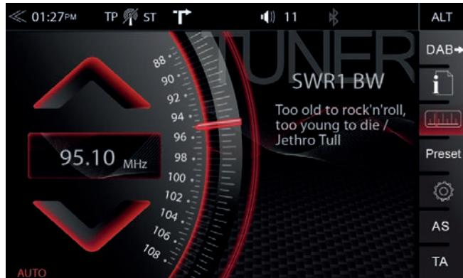
The FM setup mode (press gear icon) allows to assign two different operation modes to both station frequency arrows: manual steps in 100kHz, or auto scan (stopping at next station). See page 18.
