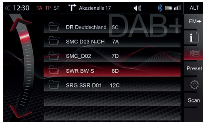
Once the first DAB+ band scan has completed, device will show all DAB+ Ensembles and radio stations of sufficient signal strength. The ensemble list and content can be updated via using the scan button.
