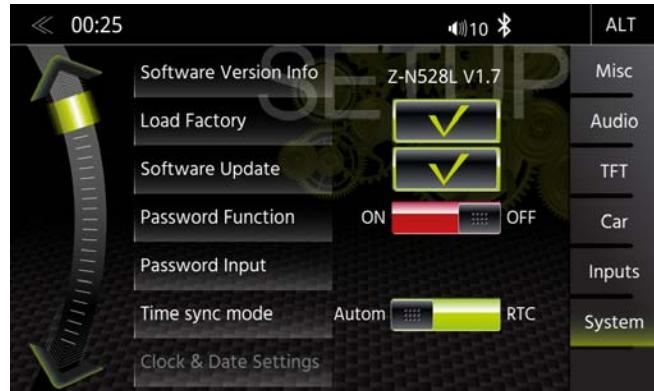
In the System Setup menu page under SW version, you will see the currently installed software versions with detailed version info for MCU, OS and AP, inclusive a simple Short Software Version.
