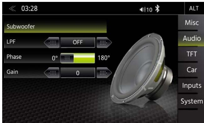
In this Expert Mode menu, you can adjust Phase, Gain, and Low-pass transition frequencies of the subwoofer. The default settings are Phase 0 °, GAIN "0", LPF OFF.
