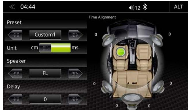
In this menu you can set the time delay correction for the loudspeakers in your vehicle.
