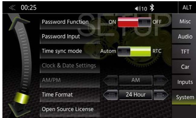
In the System Setup menu page under Clock Time, you can set the format, change the displayed time and select the time sync source (system time or autom. sync) for the time display.
