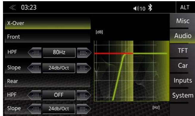
In this Expert Mode menu, you can adjust the High-pass transition frequencies of the front and rear speakers. The factory default is OFF for front and rear speakers.
