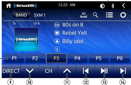
**Preset Buttons ⑧** Press and hold any preset button (1-6) to save the current station as a preset. Press the desired preset button to begin playback of the corresponding preset channel.
