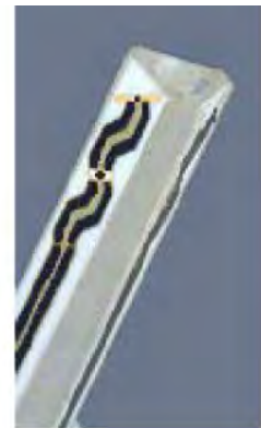
Figure 2.3 Probe Thick-Film Technique
