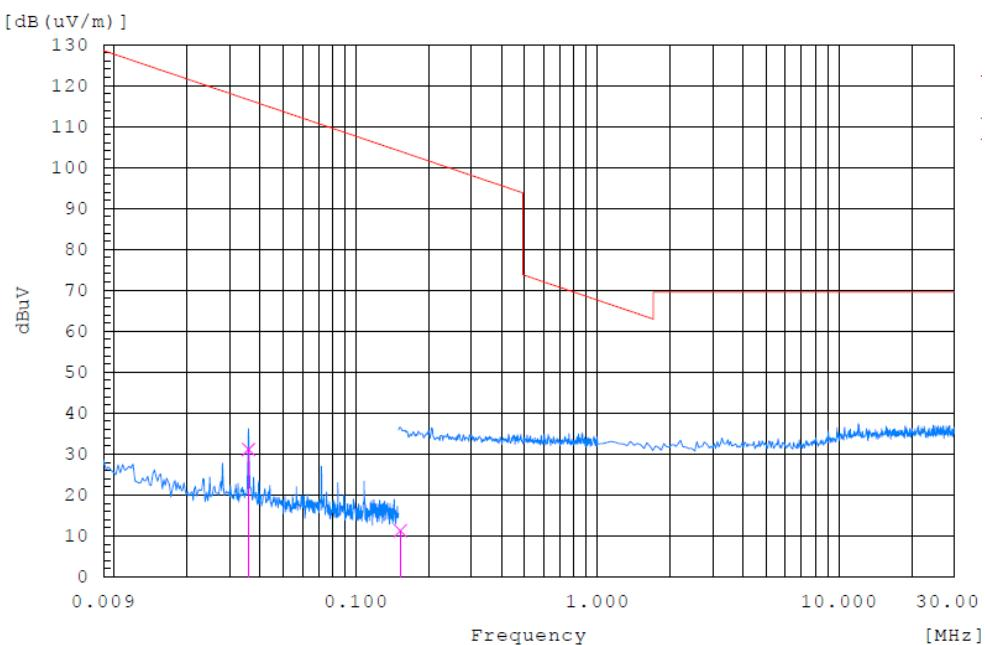
**Radiated Spurious Emission 9 kHz – 30 MHz (Antenna Position 180°)**
