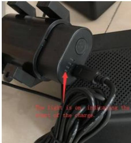
*\* This project version of the sample indicator is only used as a power-on prompt, and it won't turn off after the charge is completed. The batch version will have a full light indicator, and Bluetooth connection instructions.*
