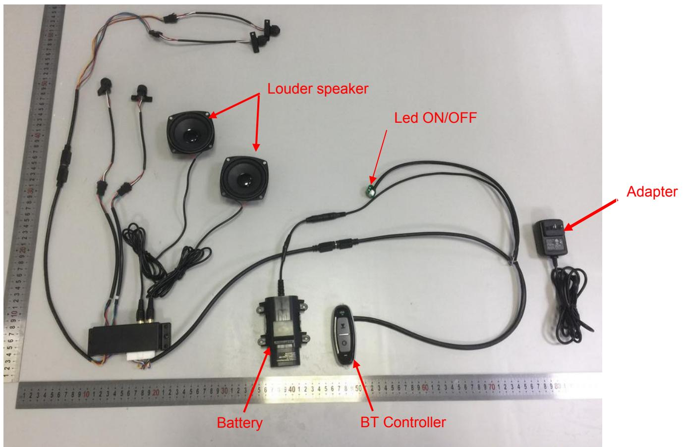
The system consists of left and right channels of high quality speakers, a Bluetooth power amplifier board, a charger, charging lines and switches. (Horn and Bluetooth power amplifier board are hidden in office chairs)
