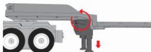
Pull out the handle and turn left to lower the bracket, Turn right to retract the bracket.
