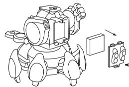
Unscrew the screw, Open the cover, and take out the battery
