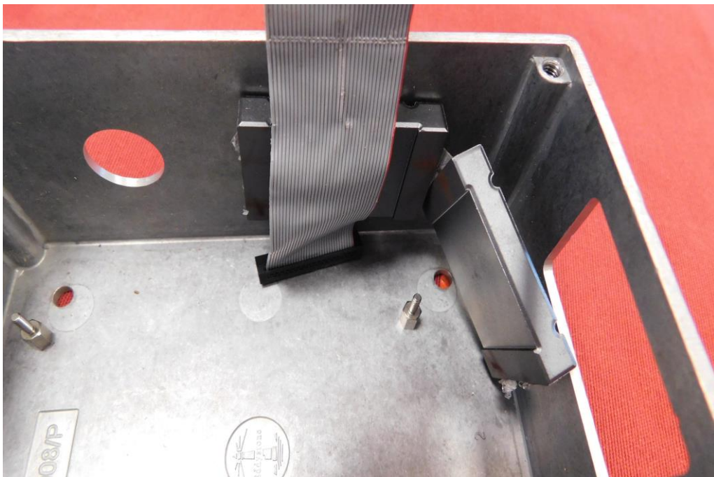
Picture 4: Detailed view of ribbon cable
