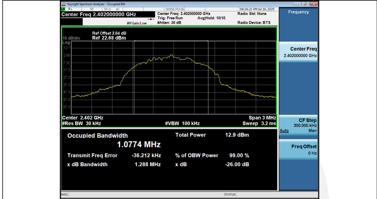
99% Occupied Bandwidth NVNT ANT1 1Mbps 2402
