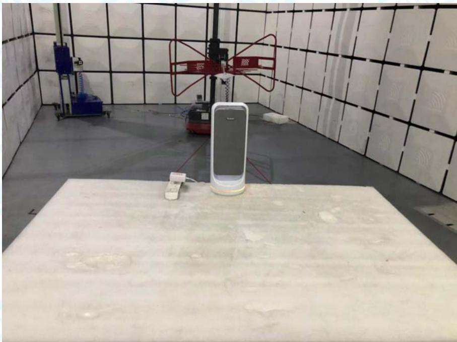
**Photo of Setup for Conducted Emission**
