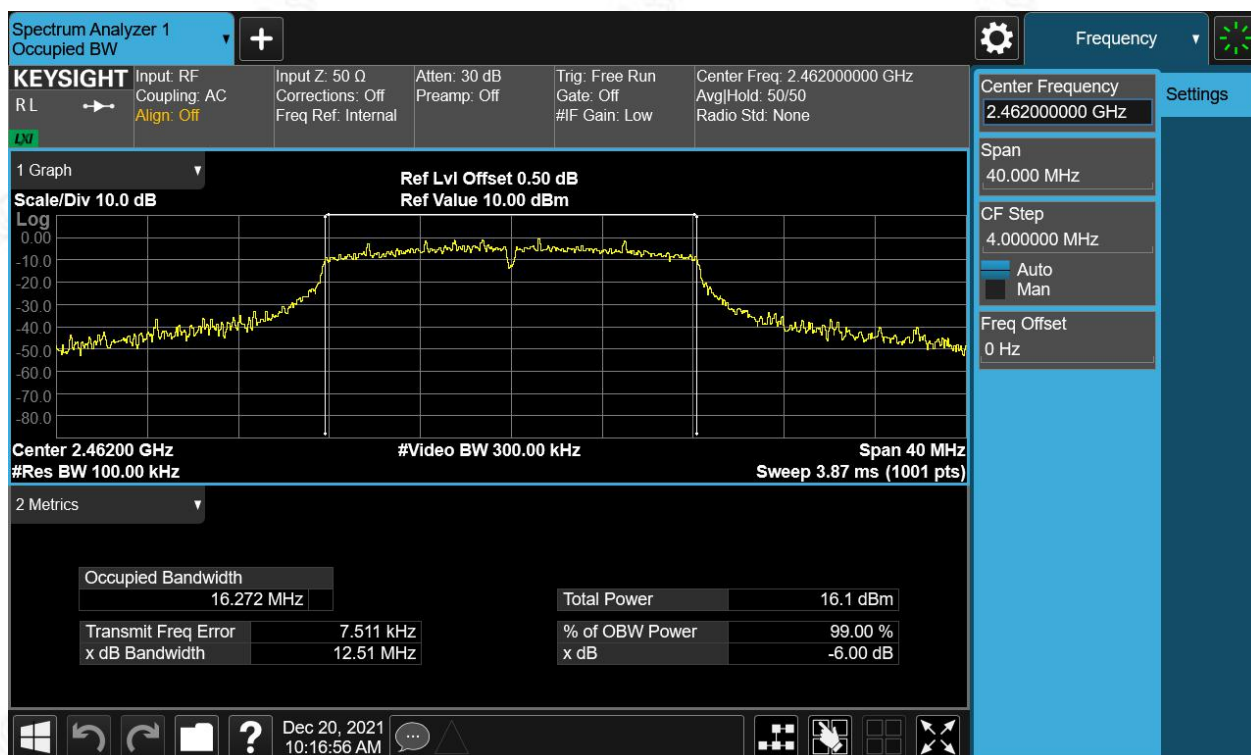
Figure 6: 6dB Bandwidth, 802.11g, 2462MHz
