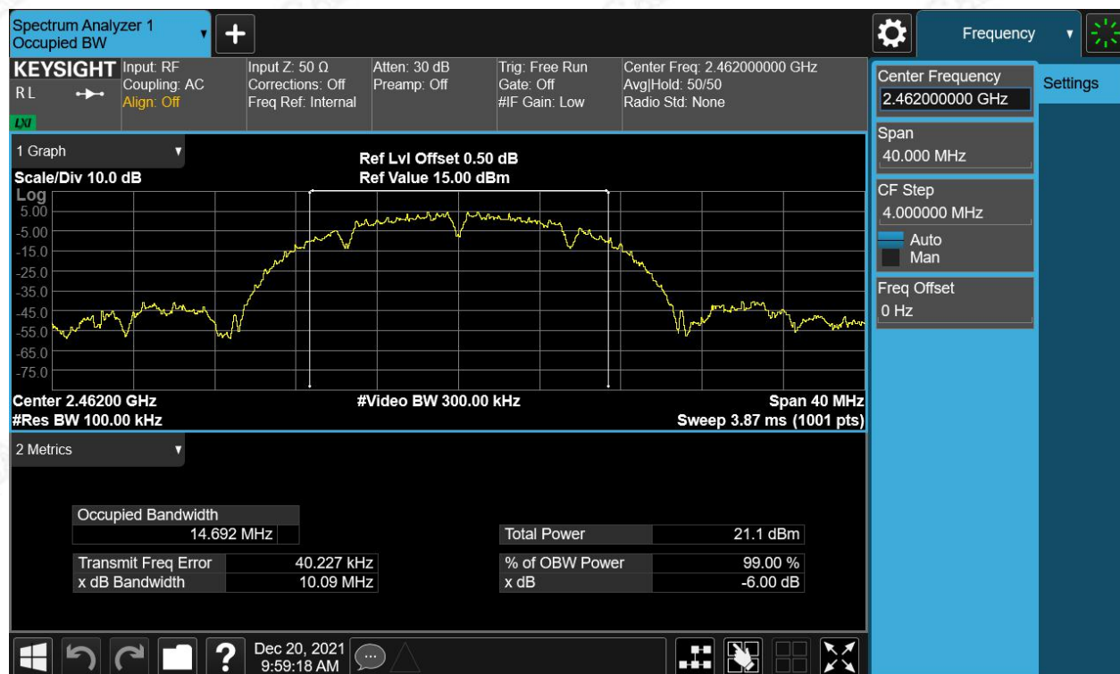
Figure 4: 6dB Bandwidth, 802.11g, 2412MHz
