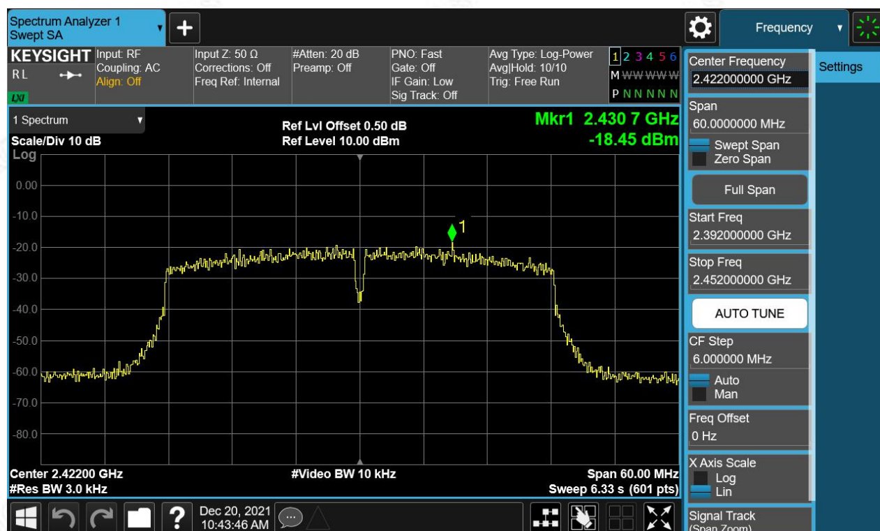
Figure 22: Power Spectral Density, 802.11n(HT40), 2422MHz
