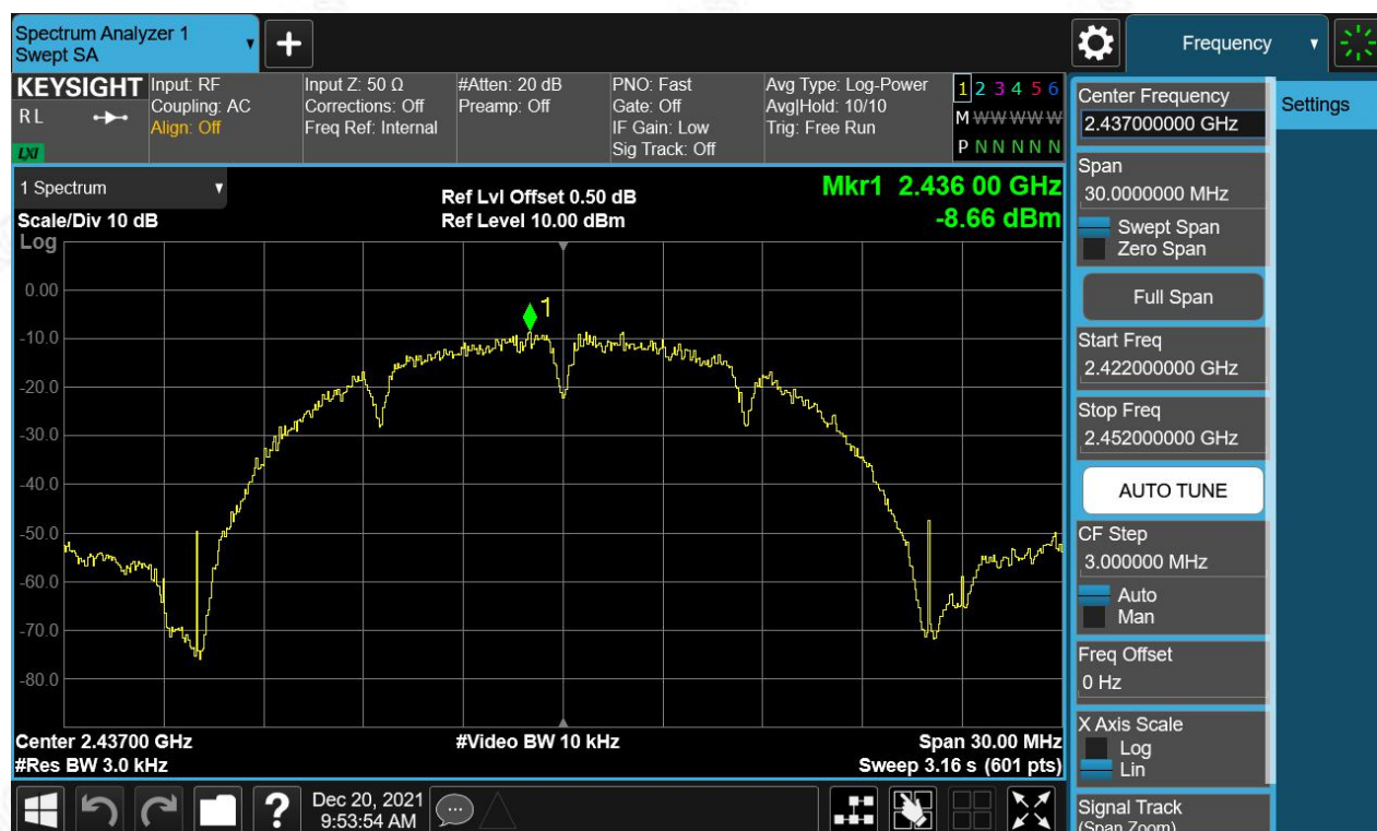
Figure 14: Power Spectral Density, 802.11b, 2437MHz
