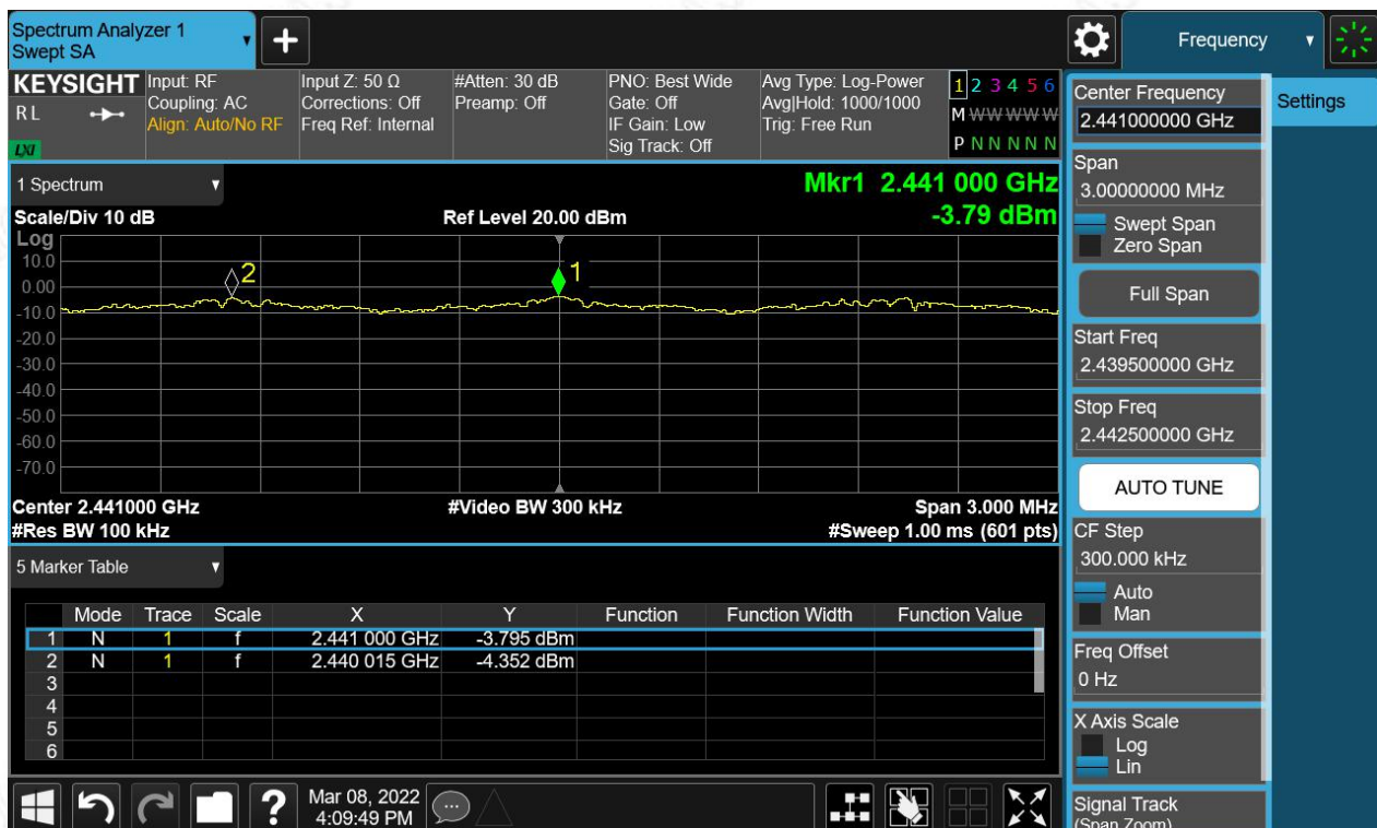
Figure 32: Hopping Frequency Separation, Hopping Mode, \pi/4 -DQPSK
