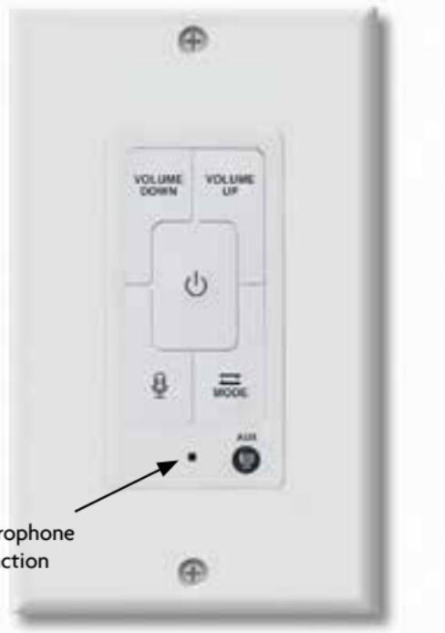
Turn the power on by pressing the center button. Center LED lit button will light in default as green which indicates it is in the WIFI mode. If the unit has the "Mode" button pressed it will toggle the mode to Bluetooth mode, which will change the center button to blue color. With the device in the WIFI mode open you will hear two audible beeps. Make sure you wait for the second audio beep. Now open the MUZO player on your device.
