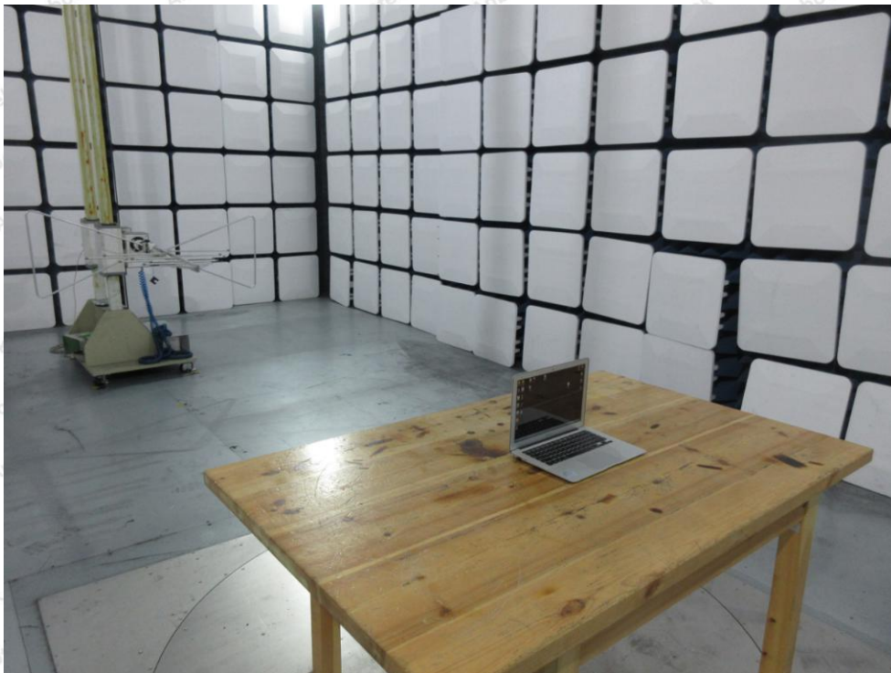
Photo of Radiation Emission Test
