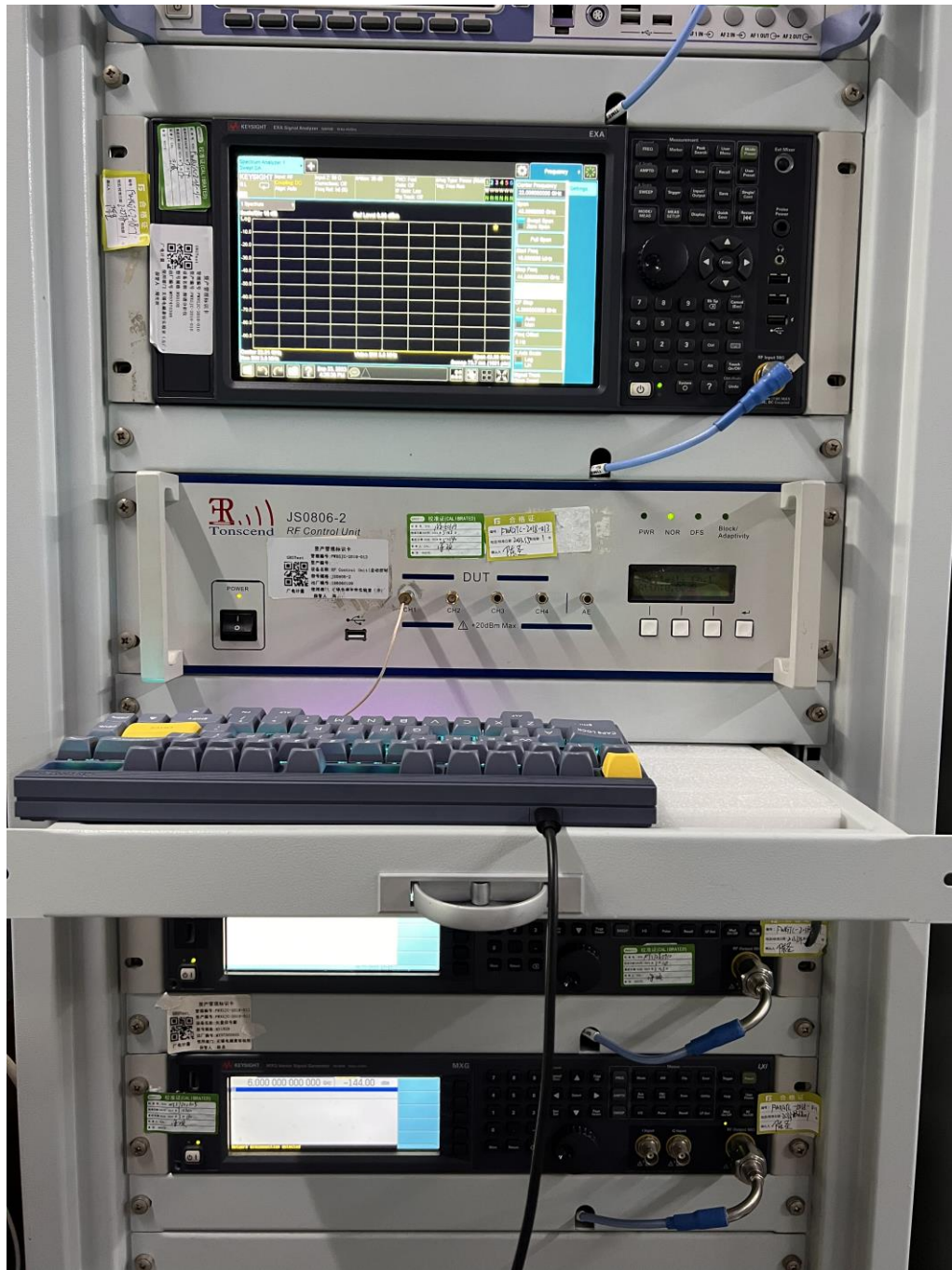
Description: Conducted Test Setup Photo
