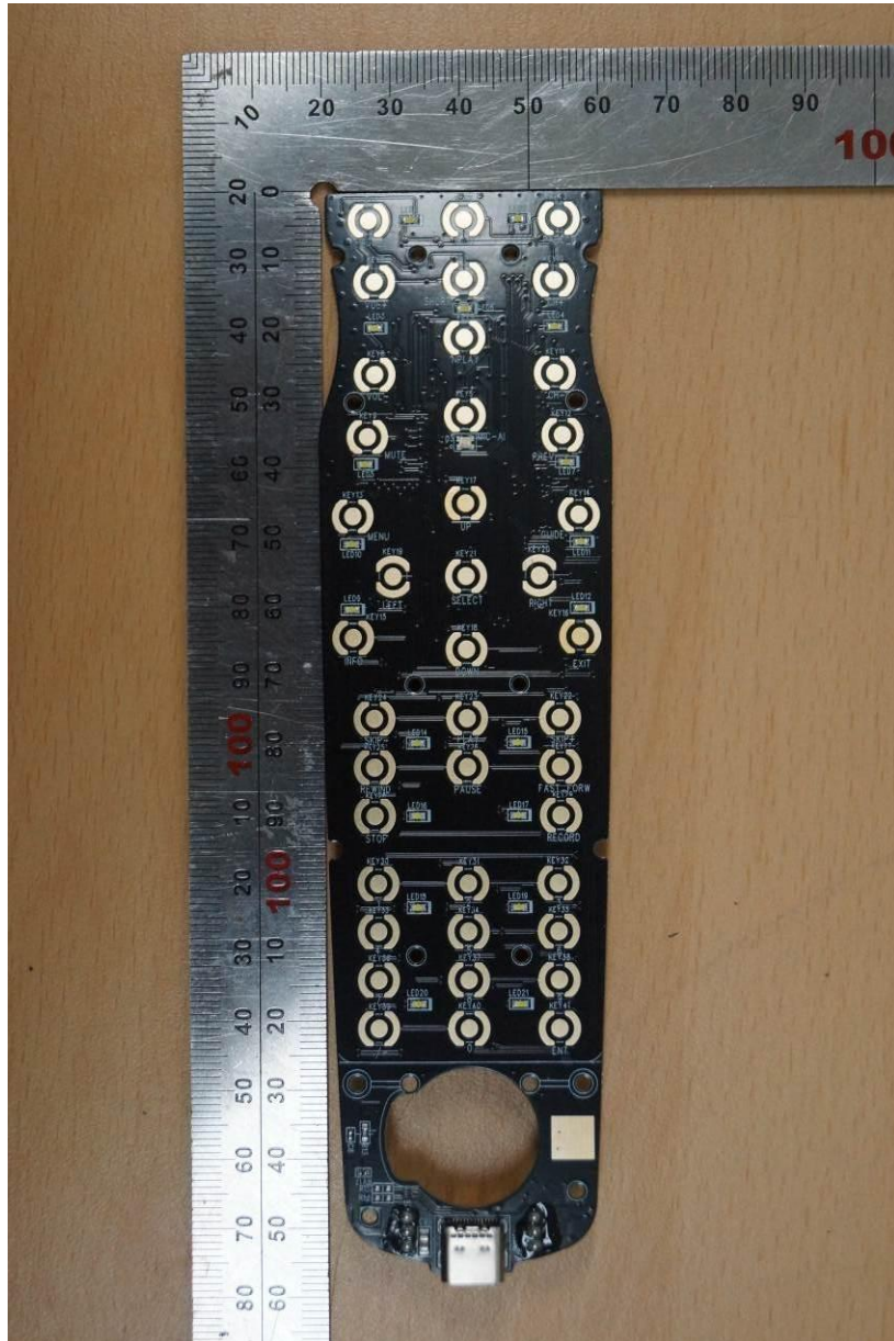
< Down-side board Top view #2 >
