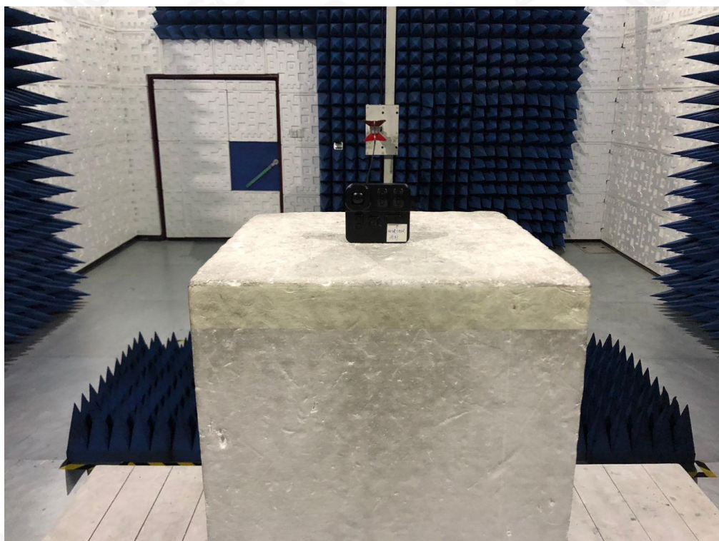
FCC RADIATED EMISSION TEST SETUP ABOVE 1GHZ
