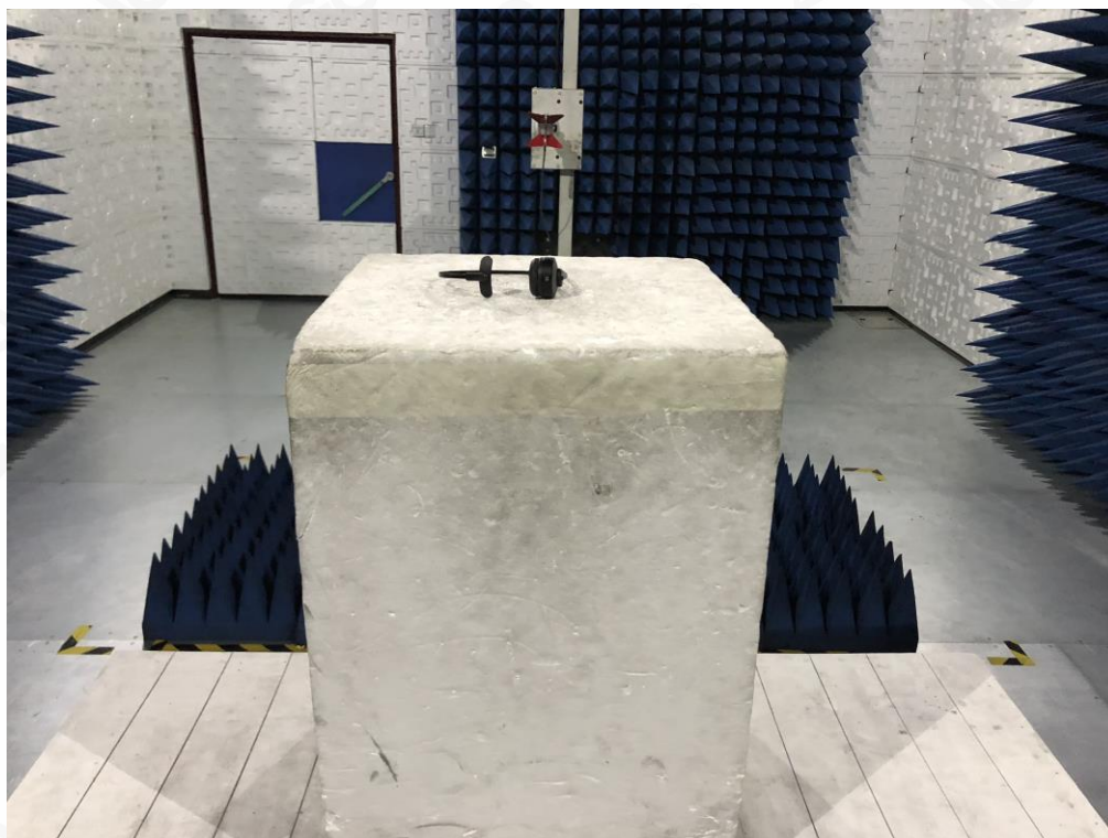
RADIATED EMISSION TEST SETUP ABOVE 1GHZ
