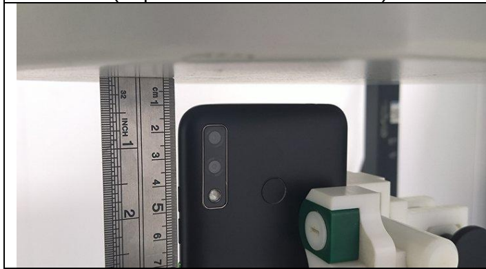
Top Side (Separation distance of 10mm)
