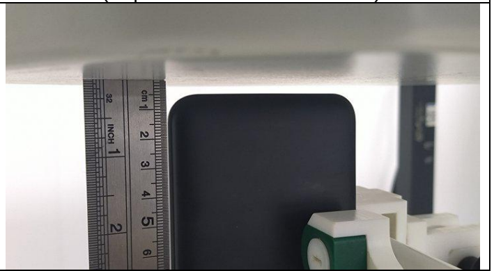
Bottom Side (Separation distance of 10mm)
