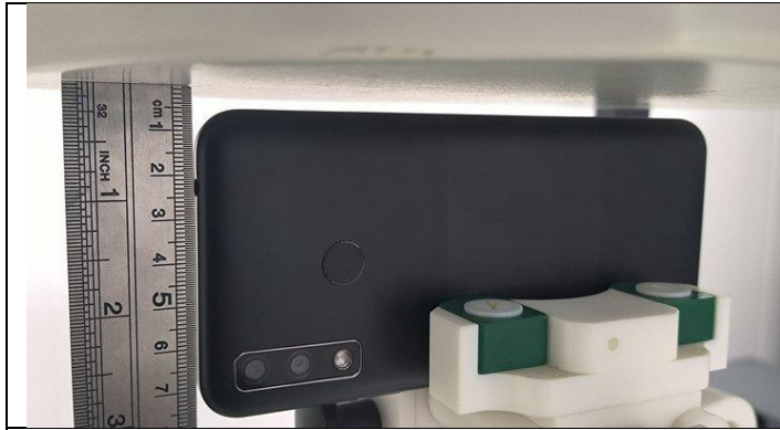
Top Side (Separation distance of 10mm)
