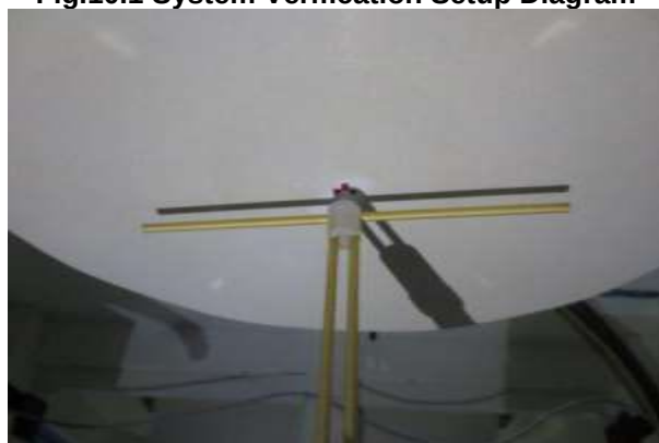
Fig.10.2 Photo of Dipole setup
