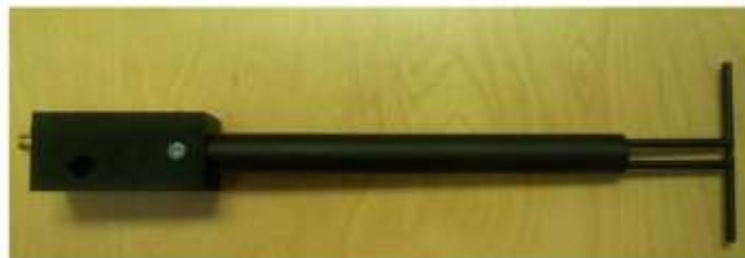
Figure 1 – MVG COMOSAR Validation Dipole
