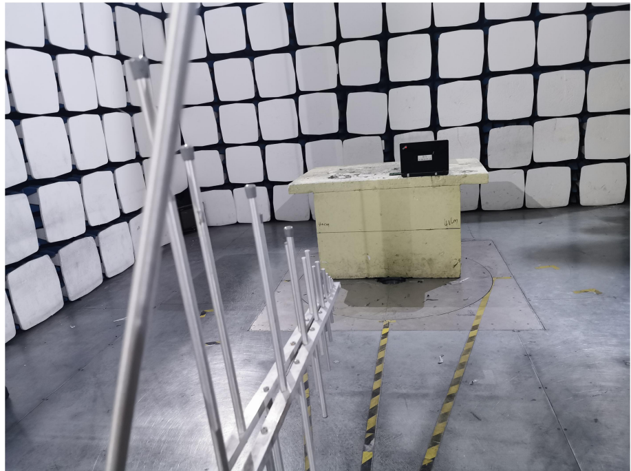
Radiation Emission Test Setup (30MHz to 1GHz)
