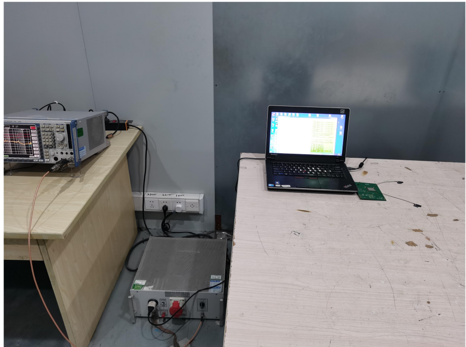
Conducted Emission Test Setup
