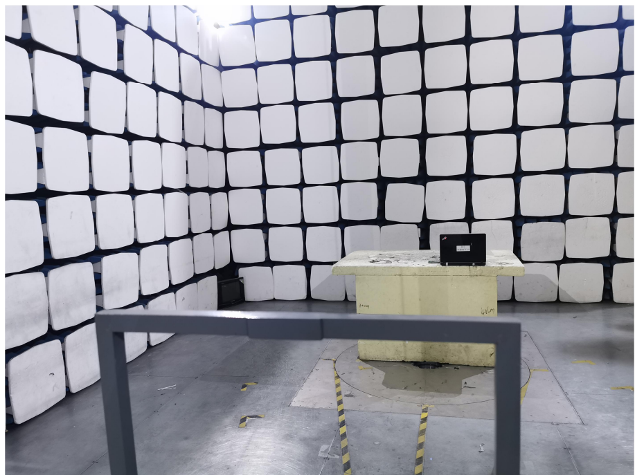
Radiation Emission Test Setup (Below 30MHz)
