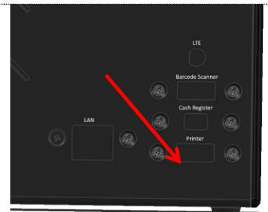
5. Connect the attached usb-cable at the cash registers usb-port and on the other side with the box using the "Cash Register" port
