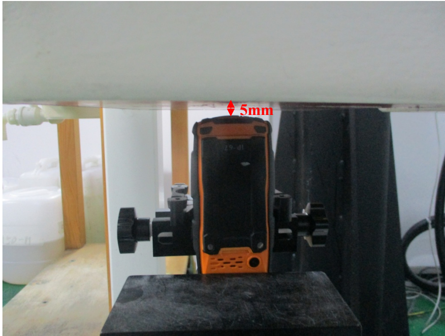
Body Bottom Setup Photo (5mm)
