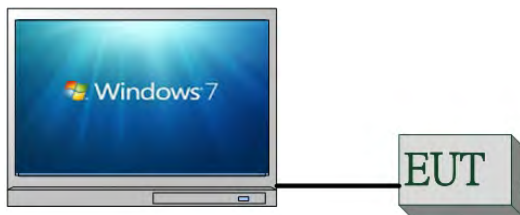
Fig. 2-1 Conducted (Antenna Port) Emission Configuration
