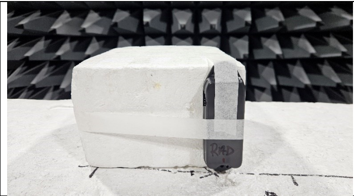
Fig B2 Test Configuration Position at 0 degrees Orientation O1 (Vertical)
