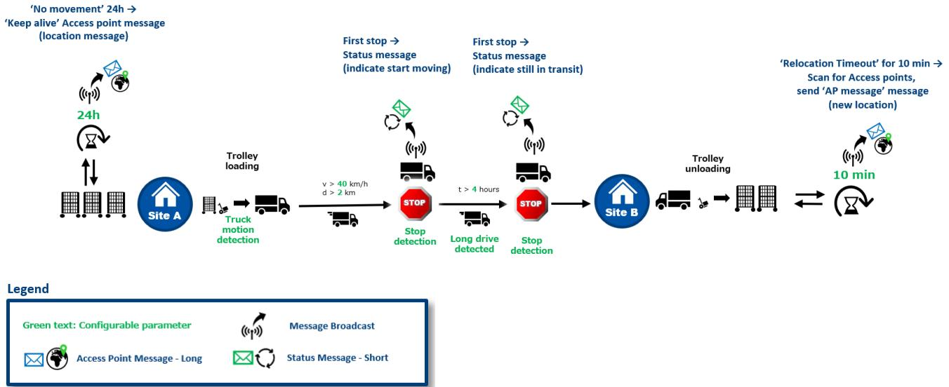
Firmware implemented according to state diagram. Note that speed and distance threshold are only estimated values and is not an absolute value, i.e., they are subjected to tolerances as actual speed is not measured by the device.
