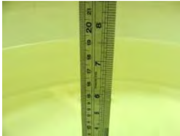
Photo of Liquid Height for Body SAR
