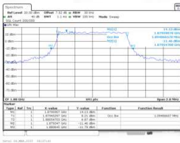
Band2 QPSK BW=1.4MHz Channel=18900 RB Size=6 Position=#0
