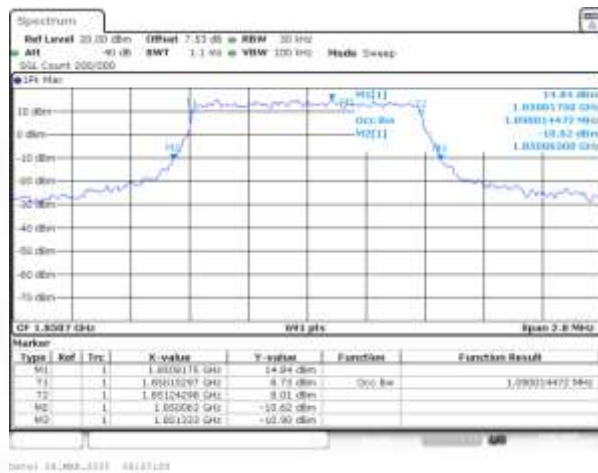
Band2 QPSK BW=1.4MHz Channel=18607 RB Size=6 Position=#0
