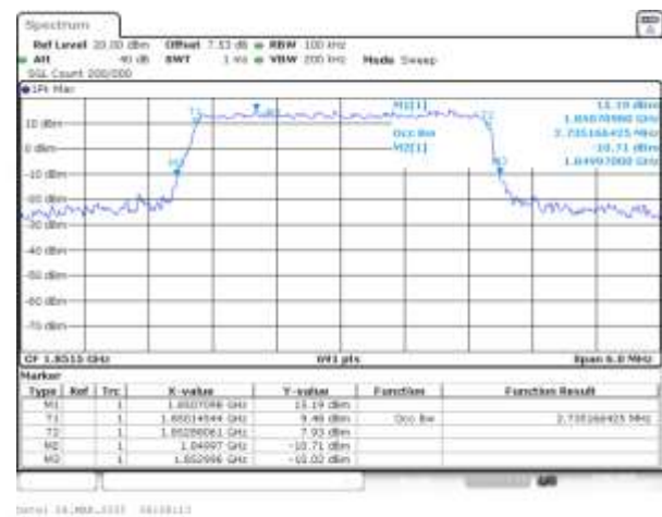
Band2 QAM16 BW=3MHz Channel=18615 RB Size=15 Position=#0
