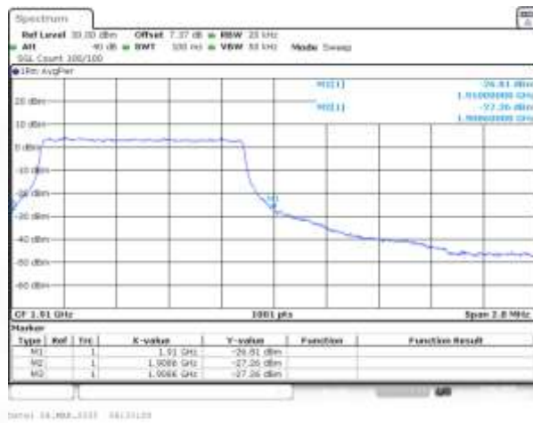
Band2 QPSK BW=1.4MHz Channel=19193 RB Size=6 Position=#0
