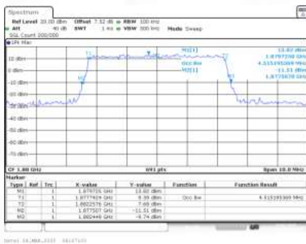
Band2 QPSK BW=5MHz Channel=18900 RB Size=25 Position=#0
