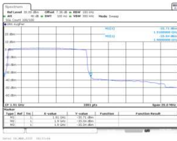
Band2 QPSK BW=10MHz Channel=19150 RB Size=50 Position=#0
