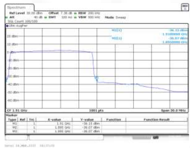
Band2 QAM16 BW=15MHz Channel=19125 RB Size=75 Position=#0
