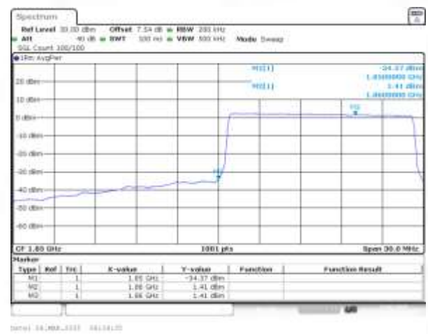
Band2 QAM16 BW=15MHz Channel=18675 RB Size=75 Position=#0
