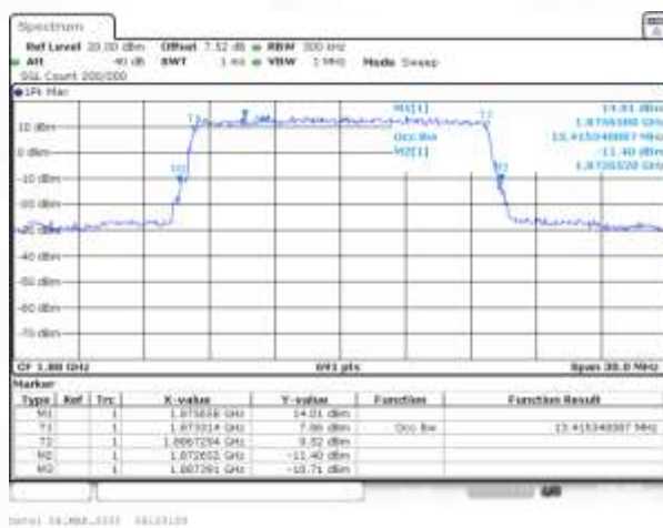
Band2 QPSK BW=15MHz Channel=18900 RB Size=75 Position=#0
