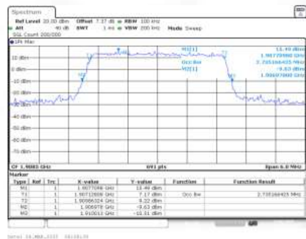
Band2 QAM16 BW=3MHz Channel=19185 RB Size=15 Position=#0
