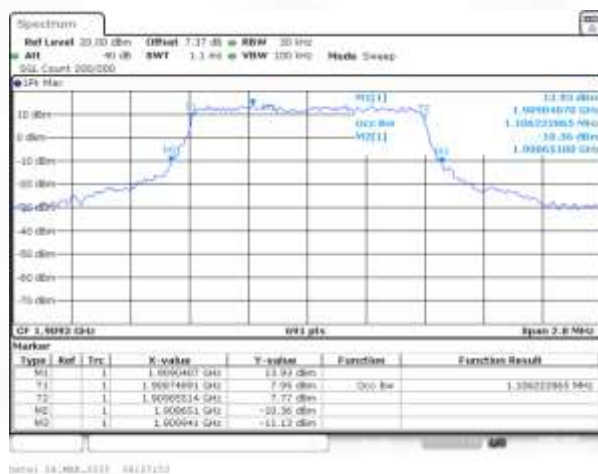
Band2 QPSK BW=1.4MHz Channel=19193 RB Size=6 Position=#0
