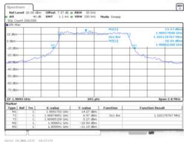
Band2 QAM16 BW=1.4MHz Channel=19193 RB Size=6 Position=#0
