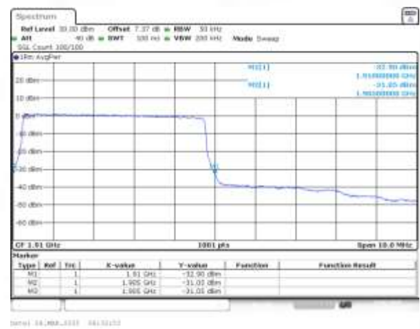
Band2 QAM16 BW=5MHz Channel=19175 RB Size=25 Position=#0
