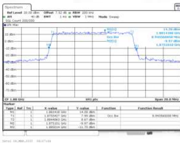
Band2 QPSK BW=10MHz Channel=18900 RB Size=50 Position=#0
