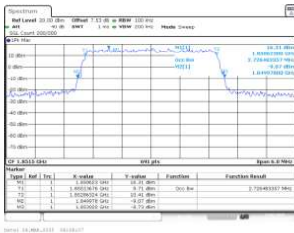
Band2 QPSK BW=3MHz Channel=18615 RB Size=15 Position=#0
