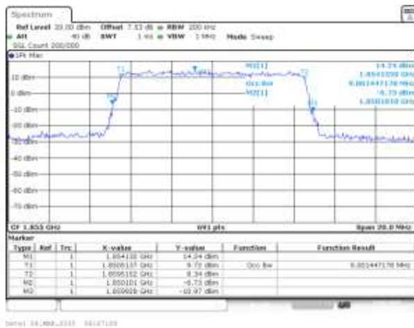
Band2 QPSK BW=10MHz Channel=18650 RB Size=50 Position=#0
