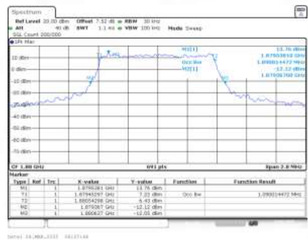
Band2 QAM16 BW=1.4MHz Channel=18900 RB Size=6 Position=#0
